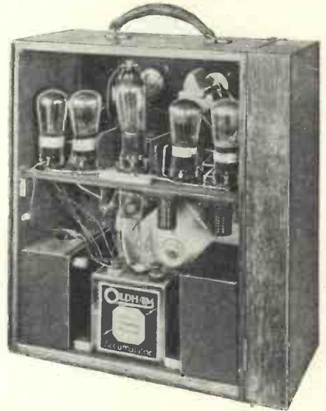
Back view of the Wayfarer, showing the positions of the batteries
