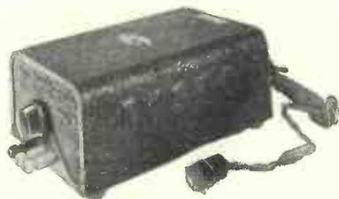
Many portables are provided with plugs so that a mains supply unit can be used for providing power, thus conserving the life of the batteries when the set is used at home extensively. This is a high-tension unit made by the Regent Radio Co., Ltd.
