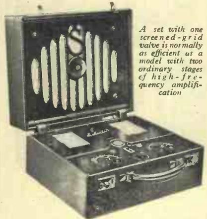
*A set with one screened-grid valve is normally as efficient as a model with two ordinary stages of high-frequency amplification*
