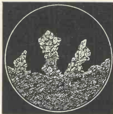
Fig. 3.—Greatly magnified view of the edge, sideways, of a terminal at the point where it contacts with an accumulator screw; showing "glassy" salt crystals due to corrosion
