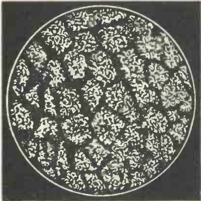
Fig. 1.—Greatly magnified view of the surface of a terminal which is in use on an accumulator. The minute grains are compact, firm, and clear yellow
