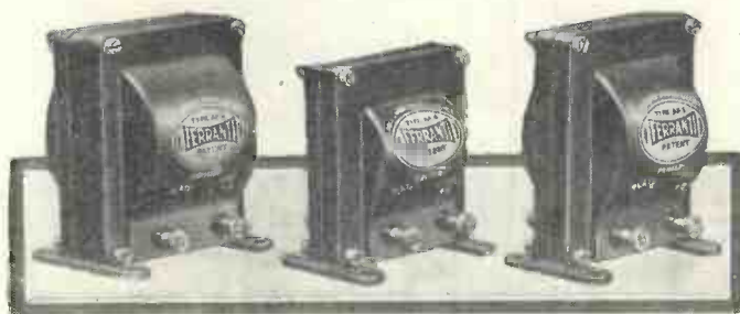
Group of three Ferranti transformers, the AF5, AF4 and AF3
