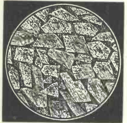
Fig. 2.—Greatly magnified view of the corroded surface of a terminal, being a relief crust of blackish green hue comprising a naked eye-view. Some parts are hard and dense; others loose
