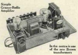
THE electrical playing of gramophone records is no new thing. For several years a valve amplifier and a loud-speaker have been employed to magnify the currents generated by an electric sound-box. But easy though it is to join a magnetic pick-up, as the electric sound-box is more usually termed, to an amplifier, there are one or two difficulties in the path of the amateur who is without the equipment necessary for measuring the working voltages and determining the characteristics of the amplifier
