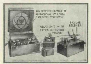
Fig. 2.—Complete apparatus for receiving wireless pictures. The cost is just over £20, exclusive of the ordinary radio set. Two models of the Fultograph are made, one in oak and the other in mahogany; each requires an extra rectifying value
