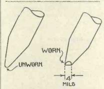
Fig. 6.—How a needle wears
