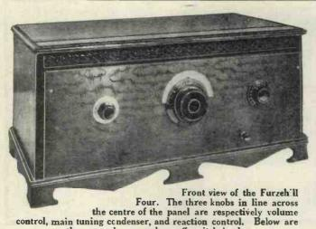
the wave-change and on-off switch knobs
