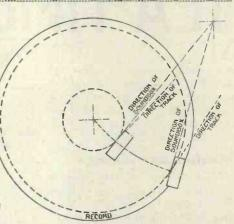
Fig. 9.—Bad needle-track alignment
