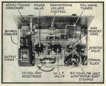
This plan view of the receiver portion of the Gramophone Three clearly shows the arrangement of all the parts. It will be seen that the wiring is exceptionally easy and will present no difficulty even to the beginner.
