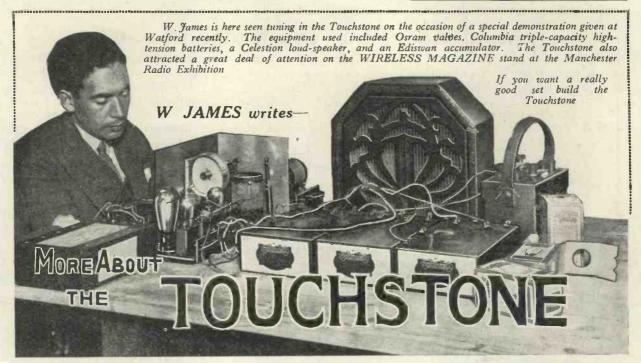
ONE of the secrets of the success of the Touchstone is the effective high-frequency amplifying stage. This really comprises two separate parts. The first is the aerial-grid high-frequency transformer which is connected to the aerial circuit and to the grid and filament of the first valve of the receiver. The second part is the intervalve high-frequency
