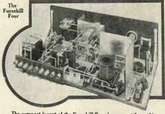
The compact layout of the Furzehill Four is apparent from this photograph, which clearly shows the arrangement of all the parts: Note especially the position of the screening
