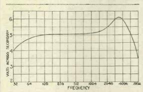
Fig. 5.—Same transformer with lower impedance valve
