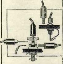
The diagram above shows the use of a spring jack attached to a socket for use with 'phone or loud-speaker tag ends or plugs. Also the
