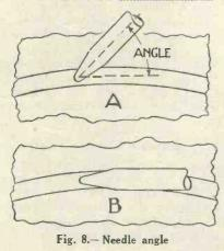
But for good playing the end should fit the groove and this is why steel needles are better than very hard ones, because the latter never wear to the groove shape. An examination under a microscope shows that an average needle covers 4 mils of length when it is worn to shape.
