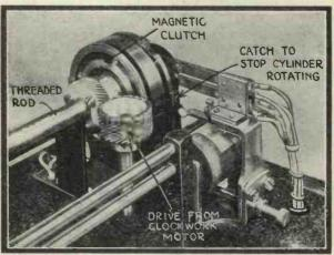
Fig. 7.—On the right can be seen the armature with its catchstop and the winding which actuates it. The threaded rod drives the cylinder and, at the same time, moves the needle carriage over the paper 1/64 in. at a time
