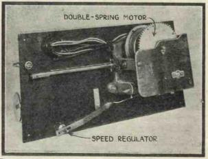
Fig. 10.—Here is another view of the double-spring motor, which is of the gramophone type. It is necessary to adjust the speed regulator so that the cylinder synchronises properly at each revolution
