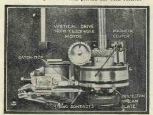
Fig. 5.—The catch-stop stops the cylinder from rotating when required and the clutch is withdrawn at the same time, thus allowing the motor to run continuously at the same speed
