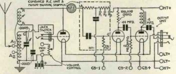
This is the circuit utilised in the Gramophone Three. The combination comprises an anode-bend detector followed by two stages of resistance-capacity coupled L.F. amplification
