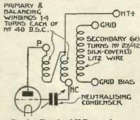
Fig. 3.—Circuit of H.F. transformer
