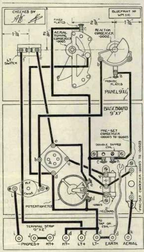
This layout and wiring diagram can be obtained for halfprice (that is, 6d., post free) if the coupon on page iii of the cover is used by December 31. Ask for No. W.M.116
