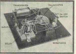
Fig. 12.—Another view of the relay unit. The transformer has a step-up ratio of 1 to 6 and is connected across the input terminals. The valve is adjusted to give a zero milliammeter reading before a connection is made to the input terminals
