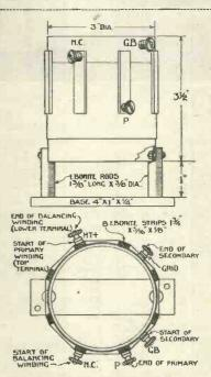
Fig. 4.—Details of intervalve H.F. transformer
