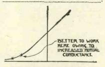
Fig, 2—Position of anode-bend point on valve characteristic
