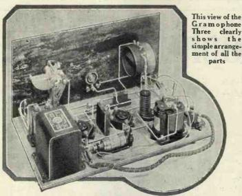
Note the all-wave tuner on the right of the panel
