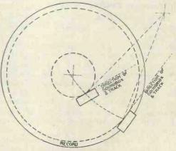
Fig. 10.-Modern needle-track alignment
