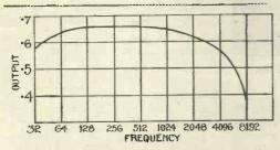
Fig. 6.—Amplification-frequency curve of Touchstone R.C. stage
