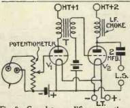
Fig. 9.—Complete amplifier connections
