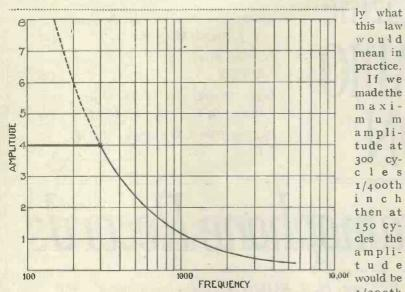
Fig. 4.—Record frequency-amplitude curve
