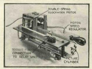
Fig. 9.—Here is the picture receiver removed from its case. The double-spring motor must be wound up for the reception of each picture, which takes four minutes to come through
