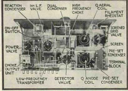
This plan view of the Furzehill Four clearly shows the layout of all the parts
