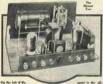
wave tuner which is provided with ten tappings and covers all wavelengths from 250 to 2,500 metres. The knob in the centre of the terminal strip is for setting the anode-bend point
