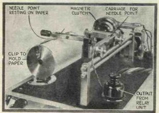
Fig. 4.—Here the needle point is seen resting in position on the paper; it is moved over the cylinder by means of a threaded rod (approximately 64 threads to the inch). The needle should be wiped after each picture has been received
