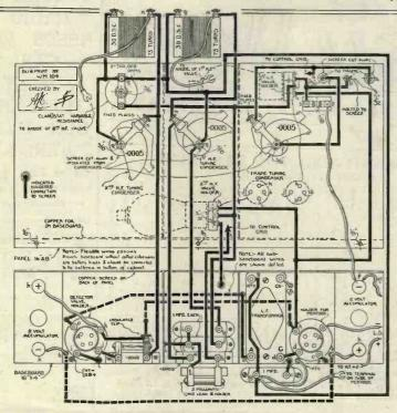
This modified layout and wiring diagram of the Super Chummy can be obtained for 1s. 6d. post free. Ask for No. W.M. 104
