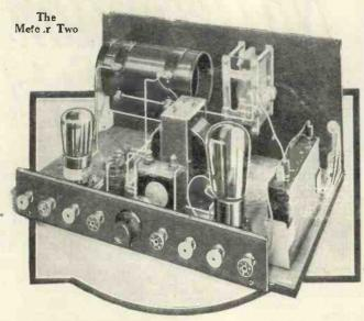
(Above) View of the Meteor Two all ready for use with valves in position. The detector is on the left and the power valve is on the right
