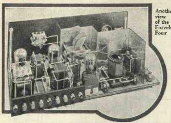
This photograph clearly shows the positions of the two low-frequency transformers and choke-capacity output unit
