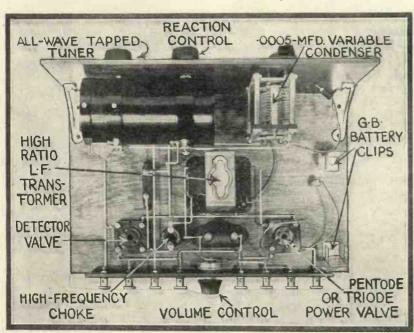
This view of the Meteor Two clearly shows the layout of the parts on the baseboard. Note that provision is normally made for a 9-volt grid-bias battery on the baseboard, but for some valves a 162-volt battery may be required
