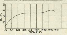
Fig. 7.—Amplification-frequency curve of Touchstone transformer stage
