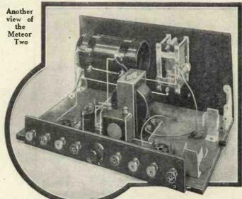
of the baseboard can be seen the 1-7 low-frequency transformer
