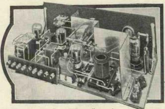
Another view of the Furzehill Four, all ready for use with the valves in position. The biassing battery for getting the best anode-bend point can be seen close to the main terminal strip
