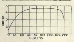
Fig. 5.-Amplification-frequency curve of the Touchstone
