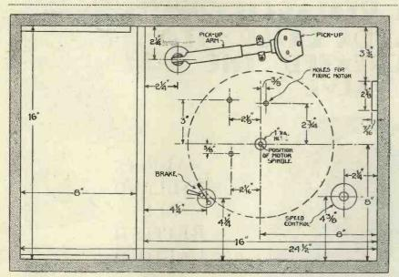
This diagram shows how the turn-table and motor, and pick-up and tone-arm, are mounted in position
