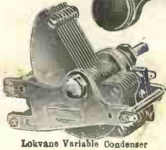
Lokvane Variable Condenser
