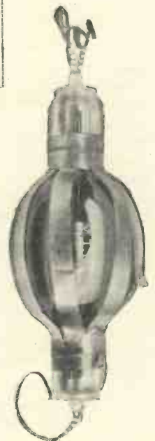
Another view of the short-wave "beam"-type apparatus used at Chelmsford is seen on the left, as is also a CAT2 oil-cooled transmitting valve. On the right is an MT10 transmitting valve.
