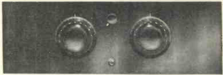
View of front panel of The Astral Four. There are two large tuning dials, for the aerial and high-frequency circuits respectively, a small reaction control, and a loud-speaker jack
