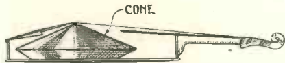
Fig. 2.—A suggested cone violin, to show how the double cone is a modified form of the violin body.
