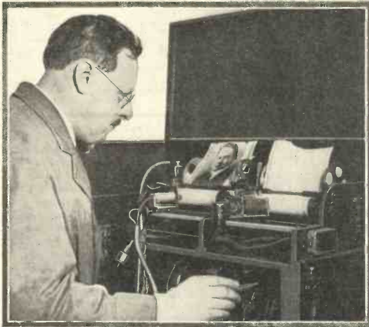
Wireless picture being received from New York by Capt. Ranger's system.
