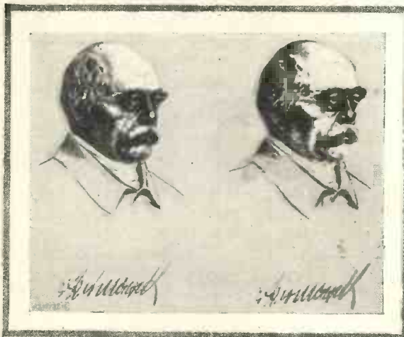
Reproductions of a photograph before and after transmission by wireless by a German system.
