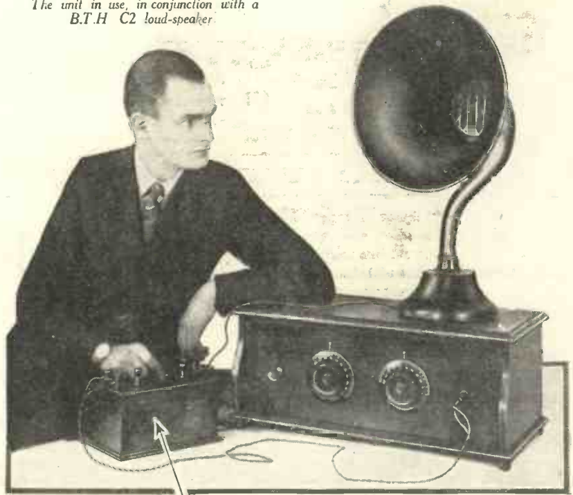
Variation in tone is obtained by operating the three push-pull switches. If desired, the adjustment can be altered for different kinds of music.
