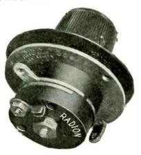
The manufacturers of the Amsco condenser have used Radion insulation in the compensator in an endeavor to keep both the surface leakage and dielectric losses at a minimum.
