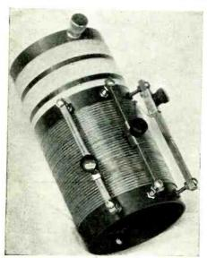
Figure 6. The complete tuning unit is shown here. Coupling between the three circuits is fixed and sliders are used to vary the inductance of the secondary
