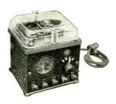
In order to make this new and complete radio battery charger harmonize with the home radio receiving set, the Valley Company has adopted a bakelite panel for the face of the charger with fittings and other parts in keeping with the use to which the instrument is to be put.
