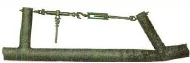
This cut, reproduced from a photograph of a test made to demonstrate the superiority of the Interlock Weld (the branch on the left) over the ordinary butt weld (the branch on the right), speaks for itself.
