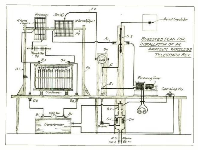
the condenser and spark gap to the primary winding of the oscillation transformer at a minimum length, the oscillation transformer is mounted on a wooden rack supported by the pillars, P-1, with the cross rod, P-2. The primary winding is permanently fixed to this rod, but the secondary winding may be slid backward and forward, thus allowing a variation of the coupling.
