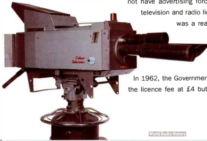
Marconi 'coffin' camera used in the BBC colour experiments at Alexandra Palace
