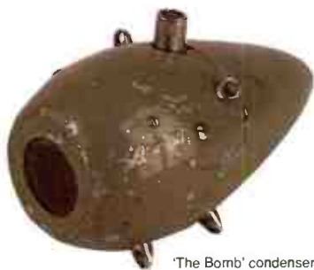
'The Bomb' condenser-type microphone, introduced in 1934
