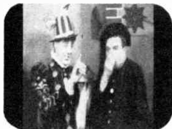
9. Picture width control requiring adjustment
