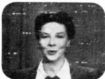
7. Effect of interference—motor vehicle ignition
