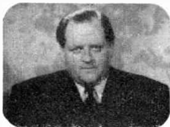
2. Effect of setting brightness control too low
