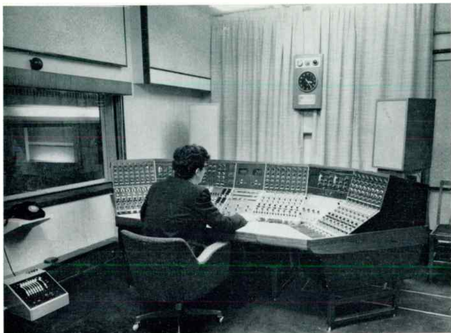
25 Stereo control cubicle in Broadcasting House, London: The studio manager faces away from the observation window, and is thus spared conflict between the visual scene and the stereo illusion he is creating
