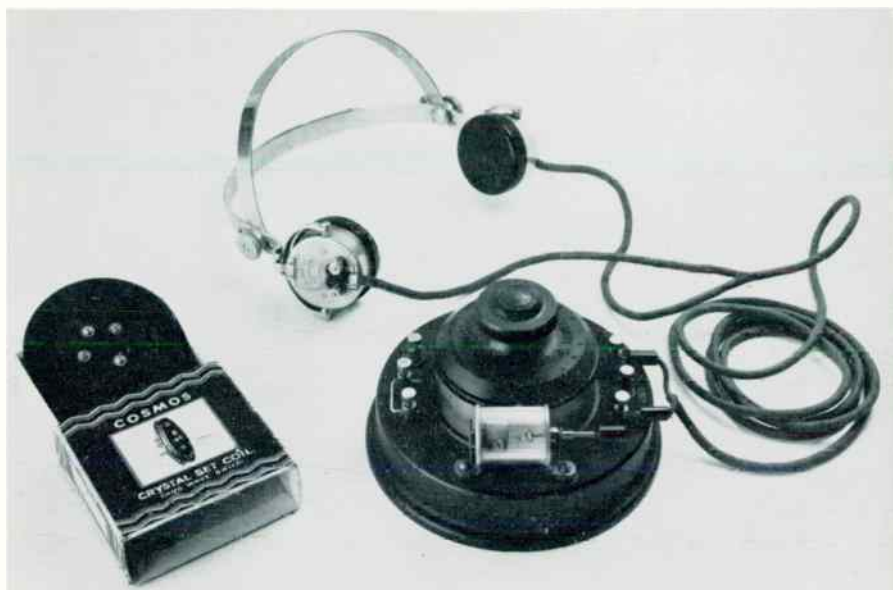
2 A crystal set of 1925: An alternative coil was plugged under the set for long-wave reception
