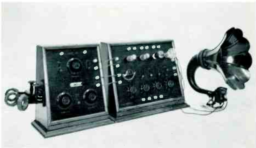
4 An early valve receiver (1923) with horn loudspeaker (1924): 'Reaction' was controlled by moving the coils at the left, and gain adjusted by switching valves in and out of circuit
