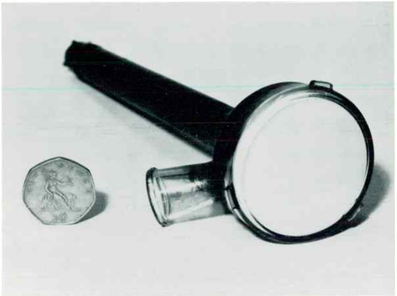
16 Projection tube, about 1950: It was possible to obtain pictures larger than the screens of contemporary picture tubes, by optically projecting onto a translucent screen an enlarged image of a small but extremely bright picture formed on the screen of a special cathode-ray tube
