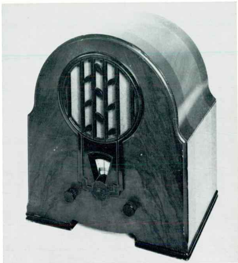
12 Philips 'Superinductance' receiver, 1933: By good design, this 'straight' set was given a performance equalling that of contemporary 'superhets'
