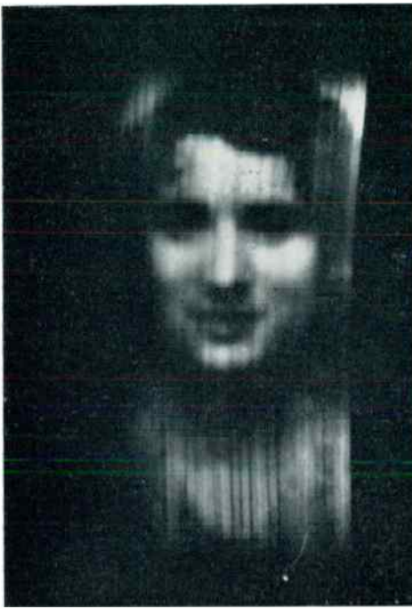
9 A 30-line television picture: As displayed on the Baird 'Televisor', the picture was enlarged by a lens to the size shown here, and had the reddish orange colour of the neon lamp employed as light source
