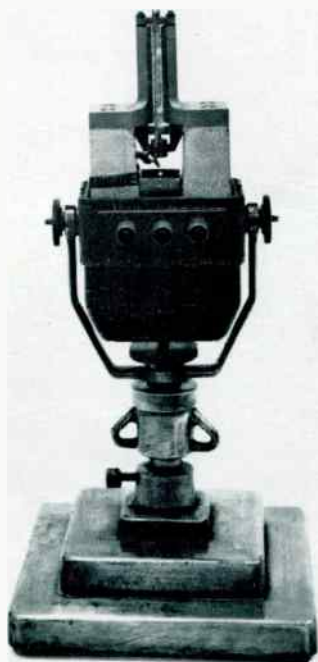
11 The BBC-Marconi ribbon microphone (1934) and an AKG capacitor microphone (1969): The earlier microphone, despite its greater size, is much less complex than the later one, which includes an amplifier employing a field-effect transistor
