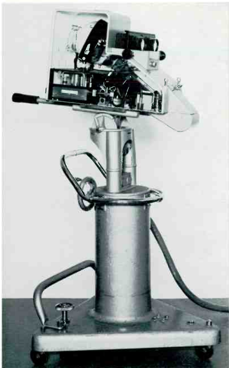
10 Emitron camera, 1936: Unlike modern camera tubes, the Emitron required the electron beam to scan the illuminated side of the 'target'; this accounts for the characteristic shape of the camera, with the electron gun protruding diagonally, below and in front of the lens. An optical viewfinder was used, in a twin-lens reflex arrangement
