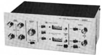
A sophisticated "black box" incorporating full Dolby B equipment for record and playback with any tape recorder. It is believed that such devices will be made and marketed in the U.K. at prices up to a little over £100. Through its use the amateur might achieve a quality standard previously obtainable only in the studio.
