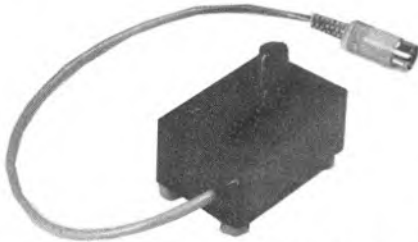
With this variable speed unit the rate of tape travel can be made to precisely equal the actual recording speed when the film was shot.
