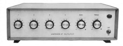
100 WATT ALL SILICON AMPLIFIER. A high quality amplifier with 8 ohms-15 ohms and 100 volt line output for A.C. Mains. Protection is given for short and open circuit output over driving and over temperature. Input 0.4v on 100K ohms.
