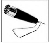
Sennheisers excellent super cardioid microphone MD411 HLM designed for the serious amateur is shown on the right. This microphone is a triple impedance unit and will therefore connect directly into any tape recorder. Frequency response 40Hz-15000Hz. A windshield is available and should be used on all exterior recordings.
