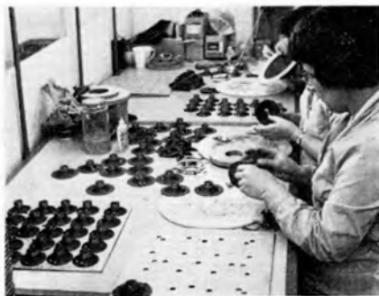
Super 3 cone assembly. Cloth surrounds are being fitted to these small tweeters. Many different kinds of adhesives are used for different stages of assembly.
