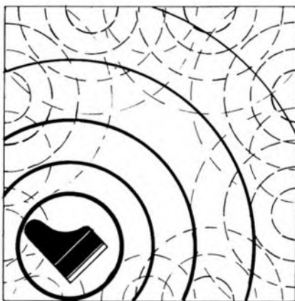
The pattern of sound waves generated by a piano in a small room or hall is very complex. Reflected sound is bounced back from all four walls as shown in the diagram, but in addition it will also rebound from the ceiling and floor. Heavy, continuous lines indicate original sound, broken lines the reflections.
