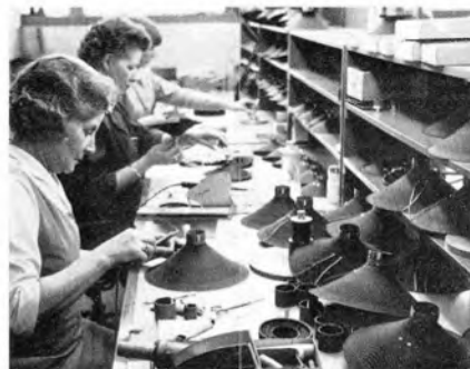
The deft fingers of long-service employee, Doris Hall, soldering pigtail leads on to 12-inch speaker cones. This delicate job requires a great deal of experience. One slip with the hot iron and the cone would be ruined. There is bound to be a great deal of repetition work in any modern factory, and the Wharfedale works are no exception. But every operative here has the opportunity of using his or her personal skills as a contribution to a product of which they are all proud. Bradford was at one time an important centre of the British textile industry. Today new techniques and new products rely upon the same gentle touch from the people who really matter—the workers on the shop floor.
