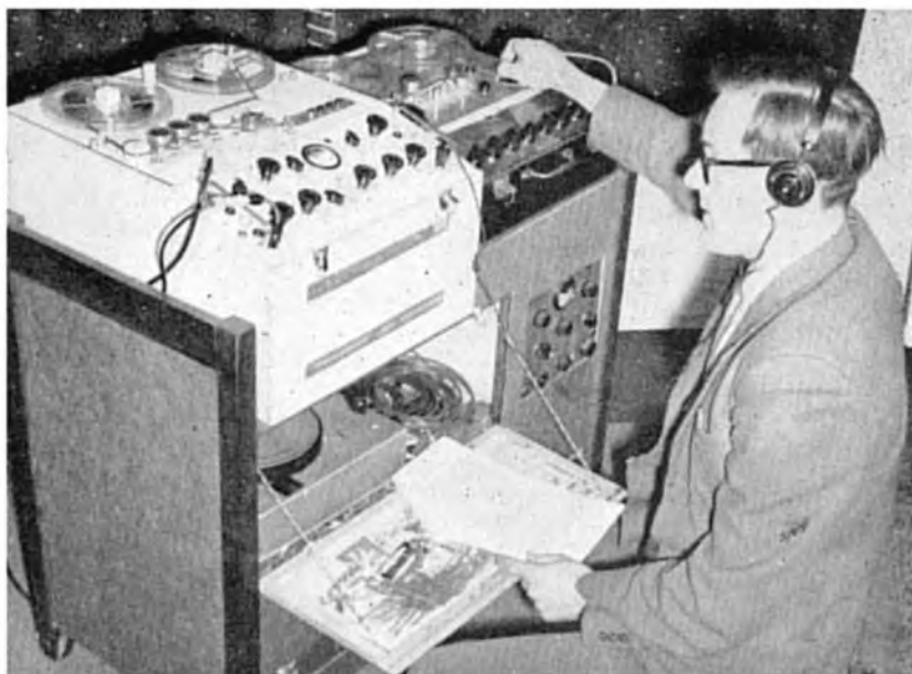
The author seen with his impressive range of equipment, all of which is carried on a trolley. In the foreground and on top is a Bradmatic deck and home-built recording and replay amplifiers (separate) with mixing facilities, contained within a single case. Beyond is a Brenell Mk V, with a Bradmatic replay head only, and pre-amplifier tone control, again in its own case. Below is a turntable and beyond that CJR record and replay pre-amplifiers. Power packs and the main output amplifier is carried in the lower space
