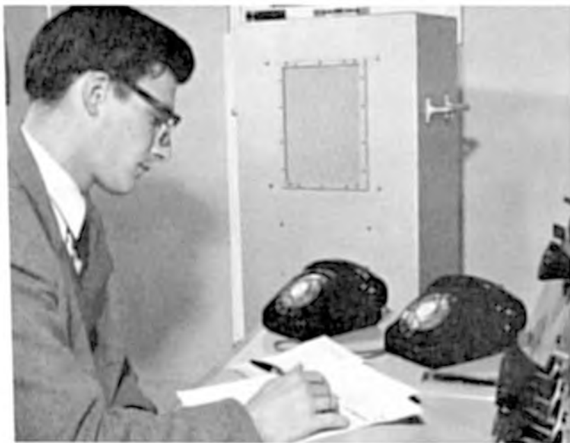
Monitoring and controlling Sports Report. Here a BBC LSU/10 is being used. This is a bass reflex system consisting basically of a twin cone unit to which a Lorentz tweeter was added to extend the h.f. response at about the time when VHF/FM broadcasts started up
