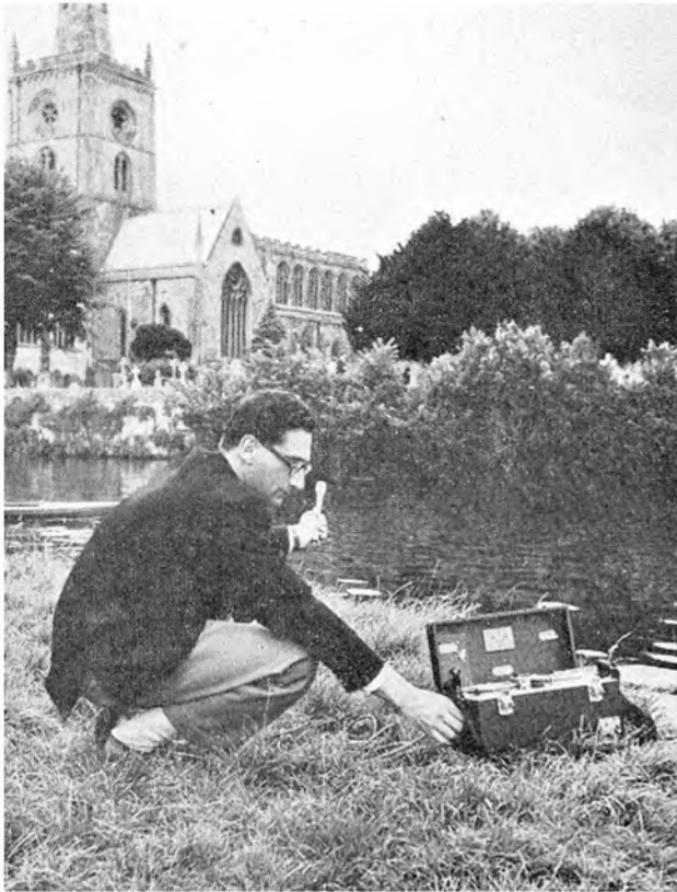
The writer recording the peal of bells of Holy Trinity Church, Stratford-upon-Avon. Equipment—Lustraphone LFV/59 moving coil microphone, Ferrograph matching transformer. EMI portable battery recorder L26. Photo by Jeremy Brownlow, Stratford-upon-Avon
