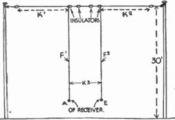
Fig. 1978.—A divided aerial:  $K^1$  and  $K^2$  are equal in length to half the wavelength,  $K^3 = 4\frac{1}{2}$  inches.
