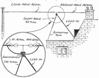
Fig. 48.—All-wave anti-interference aerial.
