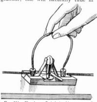
Fig. 301.—Shorting a Switch in this manner will indicate whether crackling noises are due to faulty contact.
