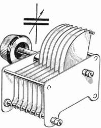
FIG. 50.—Variable condenser with air dielectric.
