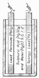
Fig. 19.—State of cell when charged.
