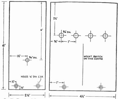
Fig. 431.—The two small Ebonite Panels. Cut from a  $7 \times 6$ -in, panel and drill as shown, the four holes in the larger piece being of suitable size for large insulated terminals. In addition the necessary mounting holes for the switch must be made on the centre line shown on the panel.
