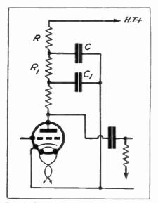
Fig. 168.—R.C.C. stage with double decoupling by resistance R and R<sup>1</sup>, C and C<sup>1</sup>,
