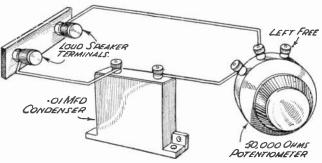
Fig. 291.-A high-note Filter-a cure for whistle, caused by hetenodyning.
