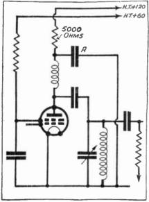
Fig. 166.—S.G. stage decoupled.
