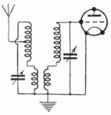
FIG. 454.—A Band-pess Tuner with common Coupling Coil.
