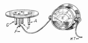
Fig. 272.—Reading the Anode Consumption of the Set in Milliamps.
