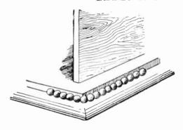
Fig. 74.—The base is improved by the addition of beading glued in the corner angle of the two parts.
