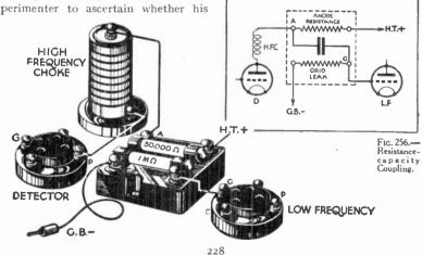
angles. Earthing the cores is very helpful, and it is also very desirable to decouple the anode circuits of both the detector and first L.F. valves.
