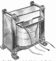
Fig. 2658.—One method of finishing off. Flexible leading-out wires are used.
