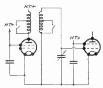
Fig. 453.—A H.F. Transformer with wave-switching.
