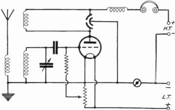
Fig. 99.—Circuit No. 2: a similar circuit to Fig. 98, employing a different system of reaction
