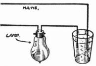
Fig. 17.—Dissolve a teaspoonful of salt in a glass of water and dip the ends of the charging wires in the solution. Bubbles of gas will form on the negative wire. (See also Figs. 26 and 27.) Take care that the two wires do not touch one another.
