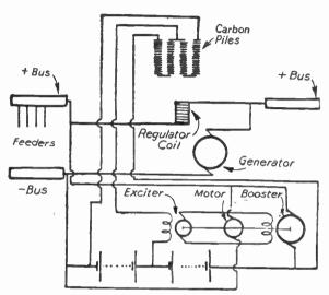
Fig. 67.—Arrangement of Automatic Reversible Booster.
