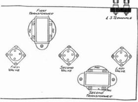
Fig. 223.—The Transformers should be mounted as far away from each other as possible to avoid interaction between them.
