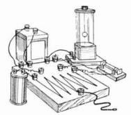
Fig. 482.—The Wheatstone Bridge and its associated apparatus.
