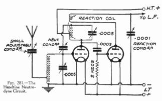
of course, but with its filament switched off. The local will probably be heard at quite good strength if the neutralising condenser is either "all in" or "all out." Adjust the neutralising condenser until the signal from the local disappears altogether. Having obtained it, move the tuning condensers slightly to make sure that it does not come in again. If it does, readjust the neutralising condenser.
