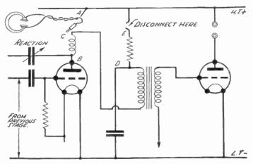
Fig. 300.—How to test for "crackling" noises. To test the H.F. and detector stages disconnect H.T. from E and join phones across A and B. To test H.F. choke as well join phones across A and C. To include transformer join them across A and D. To include decoupling resistance join across A and E.
