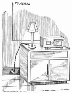
Fig. 289.—One cause of Hum is the Aerial, Earth or Speaker Leads occurs only when the set is running parallel to the Supply Mains.
