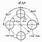
Figs. 461 and 462.—The two diagrams above show the valve-leg spacing of the Hivac midget valves (see table on page 369).
