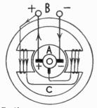
Fig. 15.—A constant voltage dynamo.
