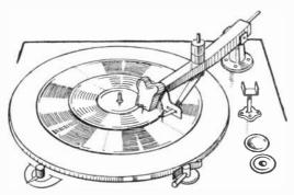
Fig. 309.—The Recorder in process of cutting a Record.
