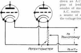
Fig. 264.-A cure for Mains Hum-a Potentiometer is connected across the Heater Supply Wiring.
