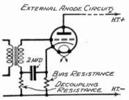
Fig. 57.—The arrangement of Fig. 56 with a Decoupling Circuit added.
