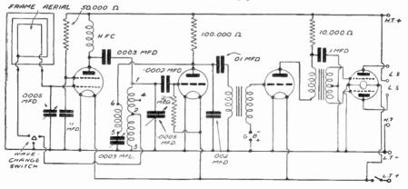
Fig. 119.—Circuit No. 21: A Four-valve Portable.
