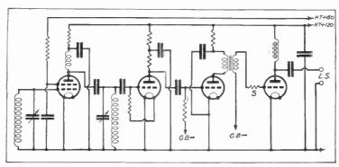
Fig. 165.—A typical four-valve circuit showing the method of inserting the decoupling resistances.
