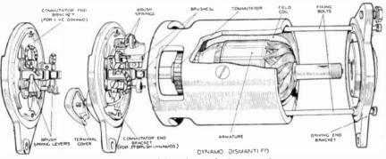
Fig. 12.-A car lighting dynamo, showing construction.
