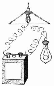
Fig. 208.—Simple Charging Arrangement from D.C. Mains.
