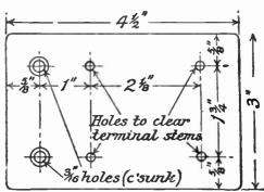
Fig. 45.—How to mark out the Ehonite Base.
