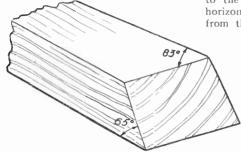
Fig. 313.—The end of the arm is cut as shown here.
