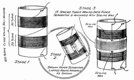
Fig. 49a.—Constructional details of the transformers for anti-interference perials.
