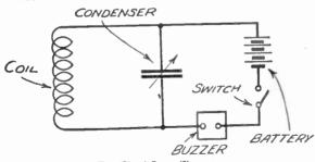
Fig. 479.-A Buzzer Wavemeter.
