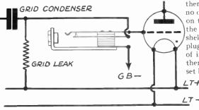
Fig. 335.—An easy way to plug in the Pick-up to the Detector Valve of a battery set.
