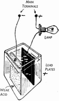
Fig. 27.—Method of testing Mains for Polarity. (See also Fig. 17.)
