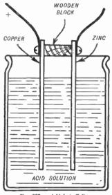
Fig. 2278.—A Voltaic Cell.
