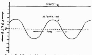
Fig. 6.—Graph illustrating difference between Direct and Alternating Current.
