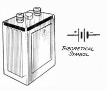
Fig. 3.—Theoretical and actual diagram of an Accumulator. Note that the thick line is always the negative in a theoretical diagram.
