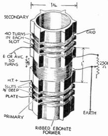
Fig. 146.—A third winding is used in this I.F. Transformer to control the degree of selectivity.
