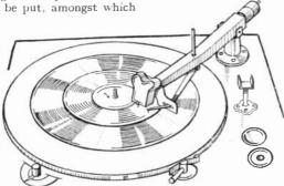
Fig. 310.—The Recorder as a reproducer. The Tracking Arm is out of action, and weights are placed on the back of the arm.
