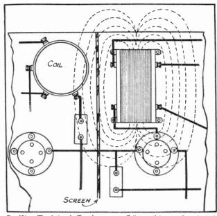
Fig. 2260.—The placing of a Transformer near a Coil (even if there is a Screen) is bad.
