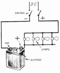
Fig. 20c.-The complete Charging Circuit.
