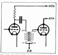
Fig. 163.—Parallel-fed Transformer. With this arrangement direct current does not pass through the primary.
