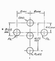
FIG. 4'8.—Valve-leg spacing for 4- and 5-pin valves. The diameter of the valve: pins is 3.2 mm.
