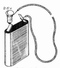
Fig. 187.-The simplest form of Tester.
