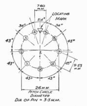
Fig. 460.—Valve-leg spating for 9-pin valves.
