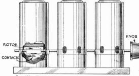
Fig. 389.—Three-gang Tuning Coil with self-contained Switch.
