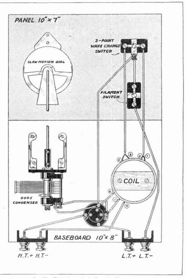
Fig. 481, -Wiring diagram for the Heterodyne Wavemeter.
