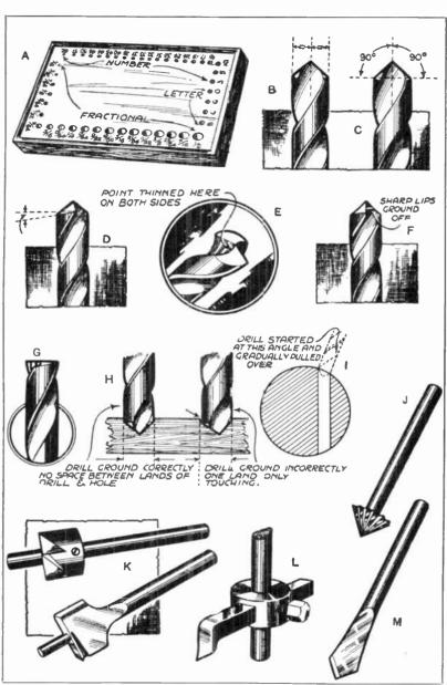
Fig. 176.-Various hines about Drills and Drilling.
