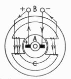
Fig. 14.—A shunt-wound 2-pole dynamo.
