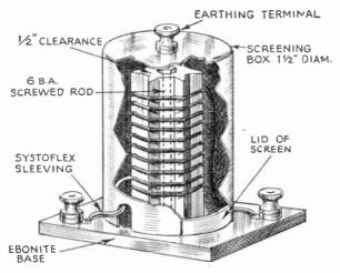
Fig. 217.—Complete assembling details of a screened H.F. Choke.
