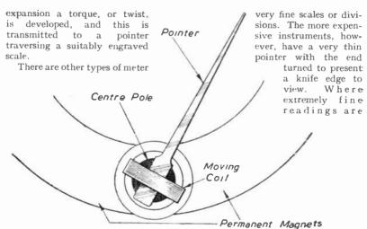
Fig. 267.—A Moving-coil Instrument with the hair spring and bearings, etc., removed to show assembly details.
