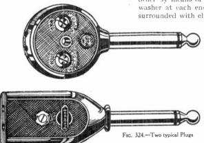
concentric and insulated from one another by means of an ebonite or fibre washer at each end. The rod is not surrounded with ebonite for its whole length, as this is unnecessary and would only add to the selfcapacity of the plug. The rod and stem аге each connected to a separate
