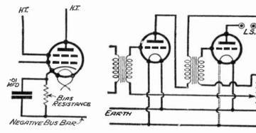
Fig. 60.—The biasing resistance arranged in the cathode lead of a S.G. valve.
