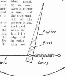
Fig. 268.—Elements of a hot-wire instrument. View showing Spring, Bearing and method of making connection.
