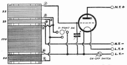
Fig. 480.—Diagram of coil connections for the Heterodyne Waverneter shown in Fig. 481.
