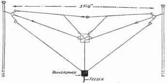
Fig. 47.—The Spider-web anti-interference aerial.
