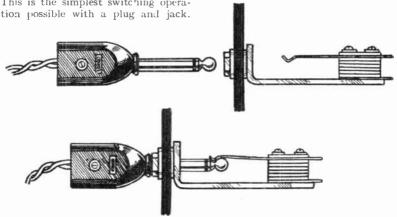
Fig. 327.—How the Plug and Jack connect.
