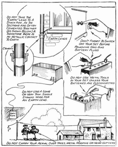
Fig. 302.—Various simple tests to apply, and causes of trouble.
