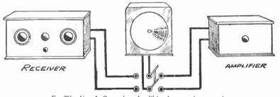
Fig. 206.—How the Gramophone Amplifying Apparatus is connected.
