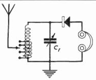
Fig. 96.--Crystal Circuit using tapped coil.
