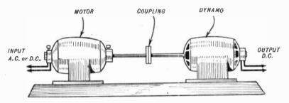
Fig. 7.—Diagram showing the principle of the Rotary Converter and Rotary Transformer. A motor, either A.C. or D.C., is driven from the mains and coupled to a D.C. generator which charges the accumulators. In practice one machine acts both as motor and dynamo.
