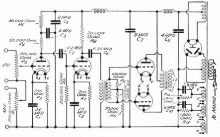
Fig. 120.-Circuit No. 22: A 12-watt Amplifier.
