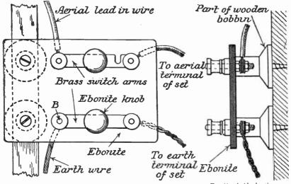
Fig. 43.-A front elevation.
