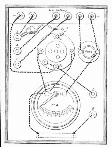
Fig. 468.—Wiring diagram of the Valve Tester.
