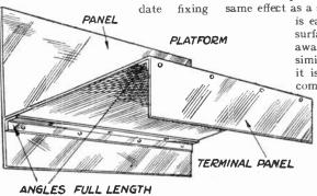
Fig. 87.—A metal Chassis using angle-irons instead of bending the aluminium.
