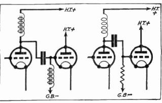
Fig. 164.—Two forms of Choke Coupling.
