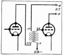
Fig. 162.—Transformer primary directly in anode circuit
