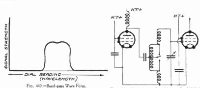
Fig. 452.—Wave-change Switching or Parallel-fed Tuned Grid Circuit.
