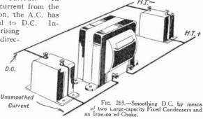
the high tension is derived for the set. Usually the inductance value of the choke is not less than 30 henries and the capacity of condensers at least 4 mfds. each.
