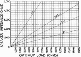
Fig. 304.—Graph for Moving-iron Speaker.
