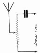
F1G. 477. —A Resistance instead of a differential Condenser in the Aerial Circuit.
