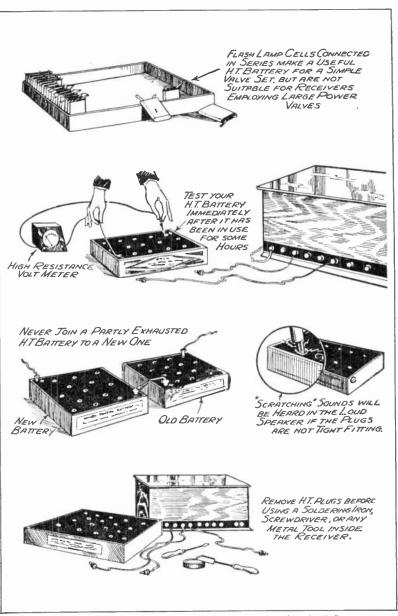
Fig. 224.—The battery user should carefully study the various points shown in this diagram.
