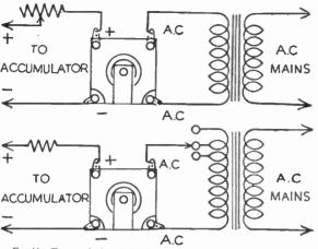
Fig. 16.—Two standard methods of employing a metal rectifier for charging
