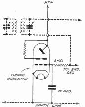
Fig. 469.—Connections for cathode-ray tuning
