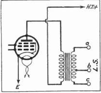
Fig. 305,-Transformer Output.
