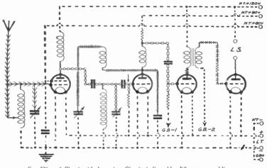
FIG. 226E.—A Circuit with the various Circuits indicated by different types of lines.
