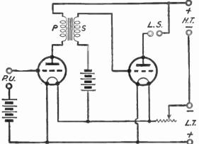
Fig. 205.—Circuit Diagram for a Two-Valve Gramophone Amplifier.
