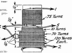
Fig. 151.—Here are the details for an oscillator coil for use with the I.F. transformer shown above.
