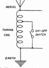
Fig. 377.--On-off Switch used for wave changing.
