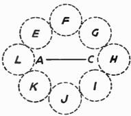
Fig. 175.—The Wave-forms of different stations approaching the frame aerial A—C.
