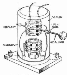
Fig. 145.—Variable selectivity is carried out in this I.F. Transformer by rotating one of the windings.
