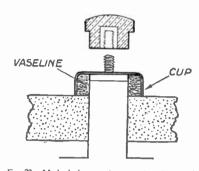
Fig. 23.—Method of preventing corrosion of terminals by means of a vaseline gland.
