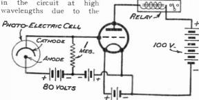
Fig. 307.—The standard method of connecting the Photo-electric Cell.
