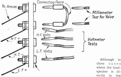
Fig. 273.—Fitting Sockets on the Panel enabling the milliammeter and voltmeter tests to be made from the exterior of the set.
