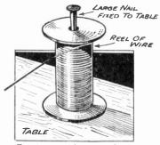
Fig. 131.—A nail driven in the bench to hold the reel while the wire is wound on the coil.
