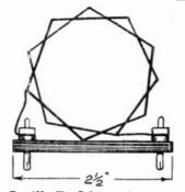
Fig. 125.—The Coil mounted on a strip of ebonite.
