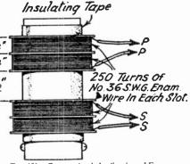
Fig. 150.—Constructional details of an I.F. transformer for 110 kc/s.
