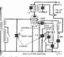
Fig. 147.—Theoretical circuit of the frequencychanging stage of a superhet receiver.
