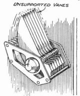
Fig. 293.—Vibrating condenser vanes may cause a microphonic howl.
