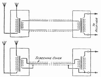
Fig. 49.—Connections for two types of impedance-matching transformer for anti-interference aerials.
