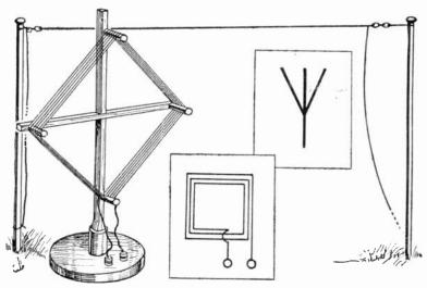
Fig. 40.—Conventional signs for outdoor and frame aerials, shown also pictorially,
