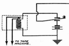
Fig. 403.—The Wiring Circuit showing how the Relay is connected.
