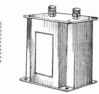
Fig. 94.—Conventional and actual diagram of two forms of L.F. Choke.
