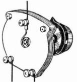
Fig. 170.—A Differential Condenser of the solid Dielectric type.
