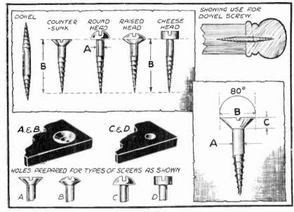
Fig. 484.—Wood Screw proportions and types.
