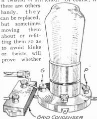
Fig. 299.—By placing the grid Condenser close to the Valve-holder the lead from Grid to Condenser is kept short—which makes for stability.
