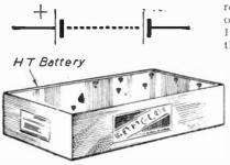
Fig. 223.—Theoretical and actual diagrams of a Hightension Battery.
