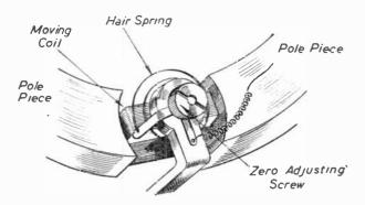
Fig. 269.—Perspective view of the active elements of a moving-coil instrument.
