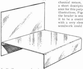
Fig. 89.—The most common form of metal Chassis. Note how the panel is holted to the front.
