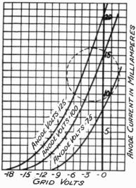
Fig. 80,—The ordinary grid-volts anode current curves.
