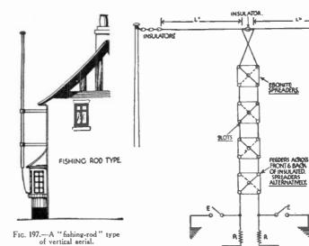
Fig. 197a.—Transposed or horizontal doublet aerial. E=earthing switches. CC=coupling coil. RR=600-ohm resistances. L¹,  $L^2$ =40-ft. aerials.
