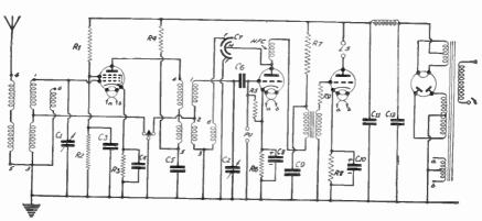
Fig. 115.—Ciscuit No. 17: A Simple Three-valve A.C. mains receiver.
