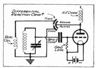
Fig. 171.—The method of connecting a differential condenser when the reaction coil is joined to the earth line.
