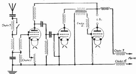
Fig. 218.—Theoretical circuit showing positions of H.F. chokes, and anti-break-through choke in aerial lead.
