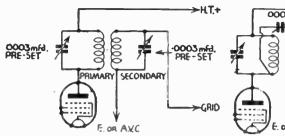
Fig. 142.-In this H.F. Transformer coupling between the two windings is carried out inductively.
