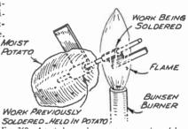
Fig. 369.—A typical case where a potato comes in useful.
