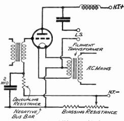
Fig. 59.—A Battery-heated Valve arranged in the same manner as Fig. 58.
