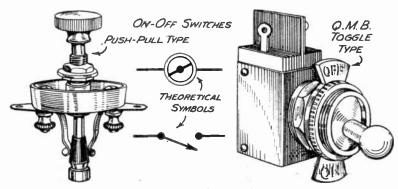
Fig. 374.—Theoretical and actual diagrams of an on-off Switch.
