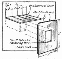
Fig. 221.—How to make the winding hobbin from paxolin sheet for chokes and transformers.
