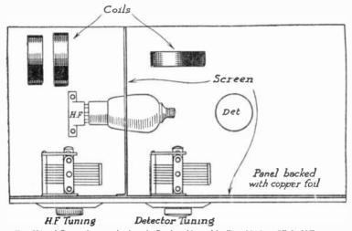
Fig. 226.-A Screen the same depth as the Basehoard is used for "partitioning off" the H.F. stage.
