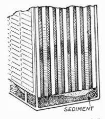
Fig. 22.—Sediment should be removed periodically, to prevent short-circuiting of plates.
