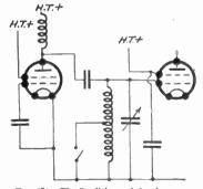
Fig. 451.—The Parallel-tuned Anode system.
