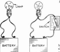
Fig. 390.—How the on-off Switch functions.
