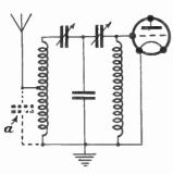
Fig. 438.—The Circuit arrangement of the Band-pass Scheme.
