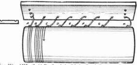
Figs. 356 and 357.—(Left) Details of the "Jockey," and (Right) the Former on which the Resistance is wound.
