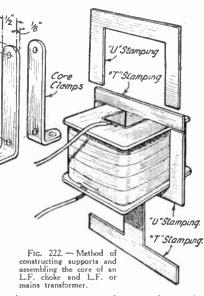
since arrangements have to be made to provide the necessary air gap. This is easily done by fitting all the "T" stampings into the spool from one end, and then arranging all the "U" stampings opposite to them. The necessary gap is fixed by slipping strips of card  $\gamma_{\sigma}$  in. thick between the ends of the "U" stampings and the sides of the "T's." Additionally, to prevent the gap being short-circuited, slips of paper must be placed between the core clamps and the core itself.
