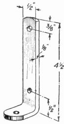
Fig. 265a.—Dimensions of supporting foot of Transformer.
