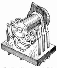
Fig. 382.—Another form of low-capacity Switch.
