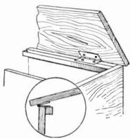
Figs. 75 and 76.—This is the simplest method of fixing the lid by means of hinges. The detail shows the extra strip for strength.
