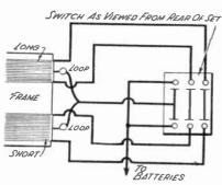
Fig. 111.—The Switch Connection to the Aerial of Circuit No. 13.
