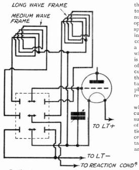
Fig. 384.—Three-pole change-over Switch used for wave changing with Frame Aenals.
