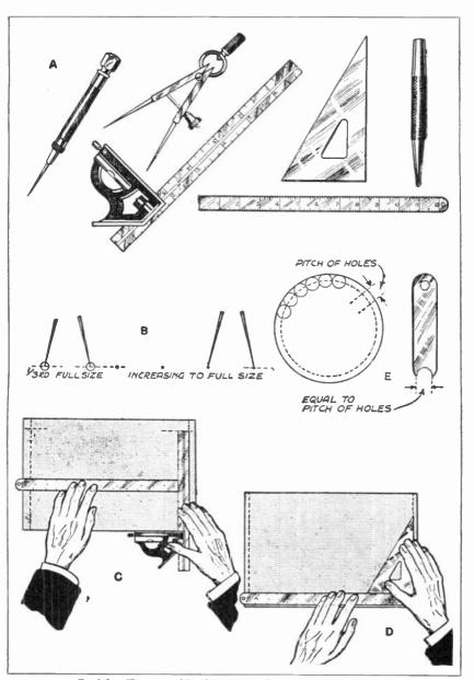
FIG. 2650.—The tools used for Marking Out, and various methods of using them.
