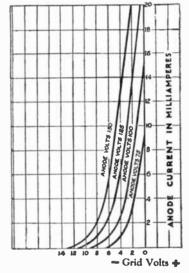
Fig. 467.—A Steep Slope Valve.
