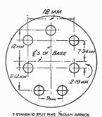
FIG. 459.—Valve-leg spacing for 7-pin valves.
