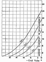
Fig. 464.—Characteristic Curve of a Low-impedance Medium-slope Valve.
