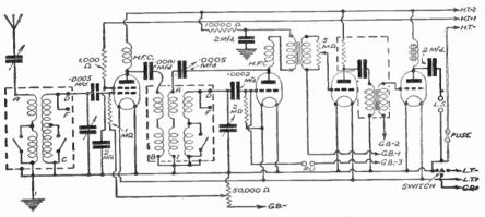
Fig. 117.-Circuit No. 19: A Simple Four-valve Battery Set.
