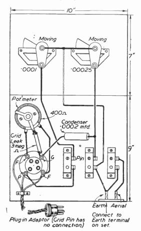
Fig. 104.—Circuit No. 7: Wiring Diagram for Short-wave Adapter Unit.
