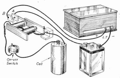
Fig. 352.—A Relay which consists of the Magnets and Armature of an electric bell.
