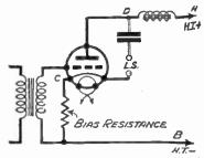
Fig. 56.—A resistance inserted in the cathode lead of an indirectly heated valve.
