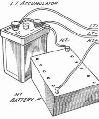
Fig. 230.—The Battery Connections.
