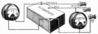
Fig. 270.-Voltmeters for rhecking different values of high tension.
