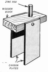
Fig. 227A.—The Carbon Plates for a Leclanché Cell.
