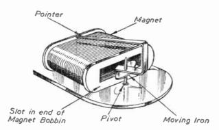
Fig. 266.—A cheap Moving-iron Movement. The top plate carrying bearing for pivot has been removed to enable the movement to be shown.
