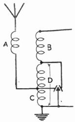
Fig. 69.—Another typical Dual-range Circuit.
