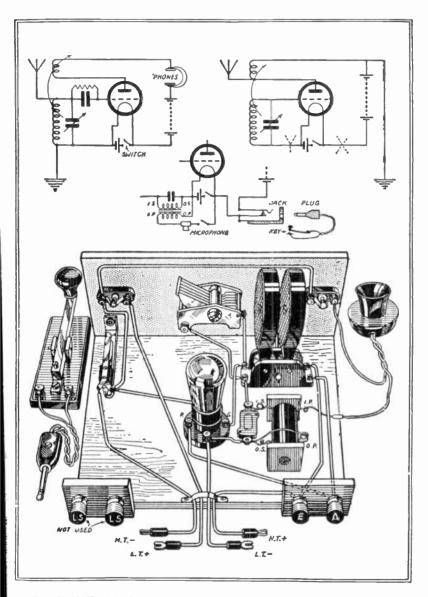
Figs. 426 and 427.—A 1-Valve Transmitter, with circuit showing how it differs from a 1-Valve Receiver. P.W.E.— M 345
