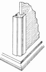
Fig. 77.—This shows plainly how corner moulding simplifies the construction.
