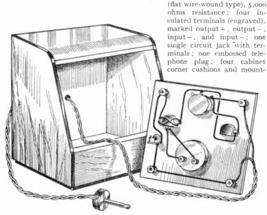
Fig. 278.—A view of the Tester with the front Panel removed to show the Wiring.
