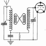
Fig. 439.—The Circuit of the "Link"
