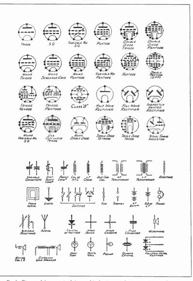
Fig. 1.—Diagram of the conventional signs used in drawing a wireless circuit, which merely consists of a number of these signs joined together. Pictorial diagrams showing the actual components represented are given in the book in their correct alphabetical order.
