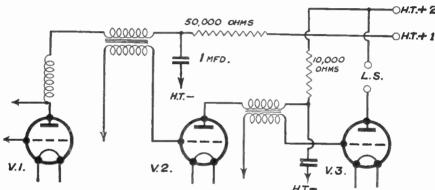
Fig. 184.—The Bettery Connections of a simple three-valver.
