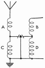
Fig. 68.—Circuit of a Dual-range Coil with which break through may occur.
