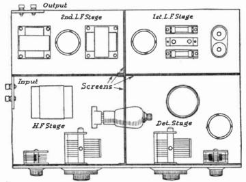
Fig. 226g.—When the Input and Output ends of the receiver come close together the set should be screened as shown.
