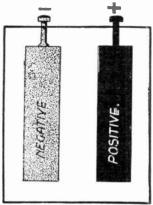
Fig. 40.—Section of a Slow Discharge type of Accumulator.
