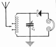
Fig. 97.—The very simplest Crystal Circuit.
