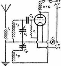
Fig. 98.-Circuit No. 1: A simple One-valve Circuit.
