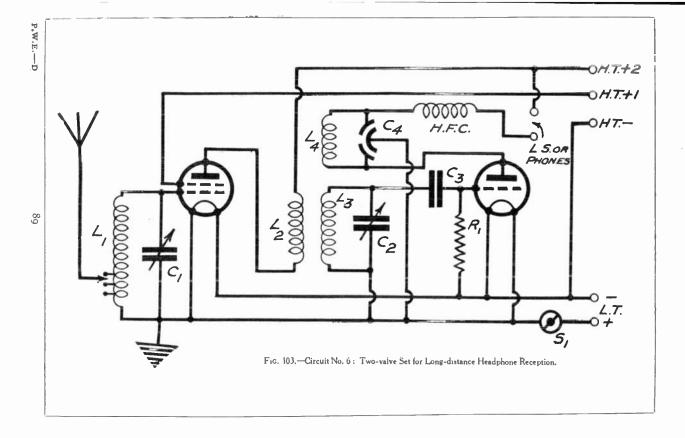
ordinary receiver (provided it is not a mains driven set), and which will enable reception to be carried out on the very shortest of wavelengths at
