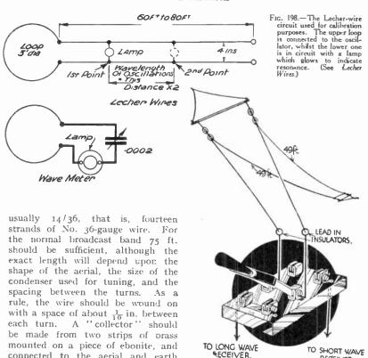
Fig. 1984.—A duplex aerial arrangement for long and short waves.
