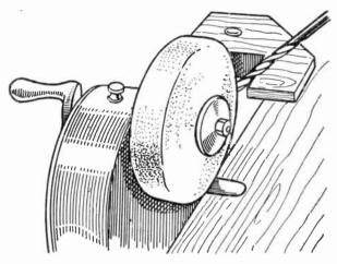
Fig. 177.—The correct angle at which to hold the Drill—and a Drill Rest.
