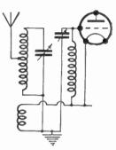
Fig. 450.—Inductive Band-pass Coupling.
