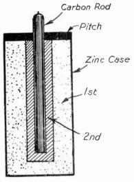
Fig. 470. - Section of a Dry Cell.
