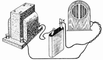
Fig. 188.—The way to test a Transformer Winding.
