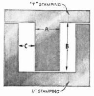
Fig. 2648.—Illustration of the Transformer Stampings to be used in conjunction with the table on p. 238.
