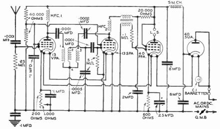
Fig. 116.—Circuit No. 18: A Universal (A.C./D.C.) Mains Three-vulver.
