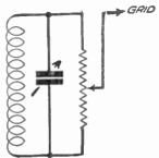
Fig. 478.—A Potentiometer across the Grid Coil.
