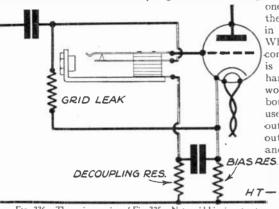
FIG. 336.—The mains version of Fig. 335. Note grid bias is cut out when the radio is in use.
