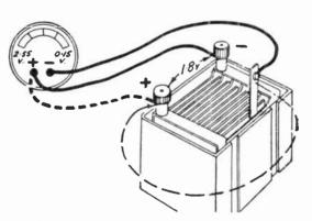
Fig. 25.—Testing a discharged Accumulator with the Cadmium Tester.
