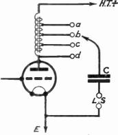
FIG. 306.—Choke-capacity Output.
