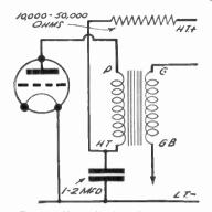
Fig. 296.—How to fit a decoupling resistance and condenser to stop motor-boating.
