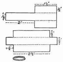
Fig. 394.—Details of the Guide Tubes through which the Tape passes.
