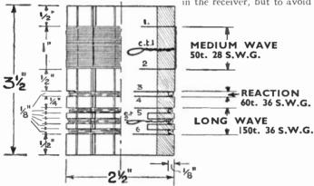
Fig. 434.—Constructional details of a Tuner made on an eight-ribbed 2½-in. diameter Ehonite Former. All turns are wound in the same direction.
