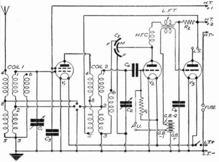
Fig. 112.—Circuit No. 14: A Beginner's Three-valve Set.
