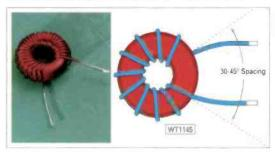
Fig. 1: Winding a toroid - spacing of the wire endings is important (see text).
