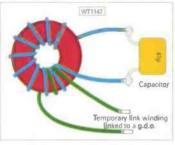
Fig. 3: The G3RJV method for checking the resonant frequency of a toroidial inductance using a dip meter (see text
