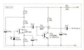
Fig. 3: A low noise laser receiver front end for night-time use, courtesy of John Yurek K3PGP.
