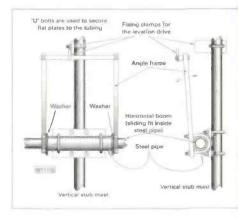
Fig. 3b: This system again uses a simple sliding-fit pivot, but this time driven by an extension arm drive, which may be cheaper and easier to set up than the system of Fig. 3a.
