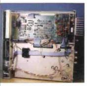
Fig. 3: The inside of the Patcomm PC-16000. showing the heatsink on the right-hand side.
