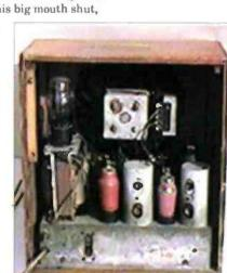
Fig. 3: Inside view of the 'Utility' receiver.
