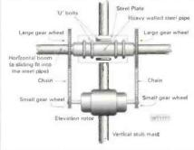
Fig. 3a: Utilising a simple sliding-fit bearing (as explained in text) and chain wheel reduction gearing a small elevation rotator can elevate quite a large antenna array such as the 'H' frame of Fig. 2.
