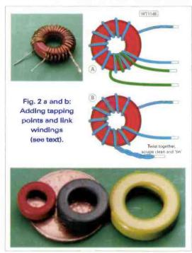
mixture or the permeability of the core. Powdered iron cores have coloured paint on one side to show the material mix but ferrite cores are all black. Usually the average constructor normally relies on the given circuit or design for choosing the core material and the designer simply tells us what to use.
