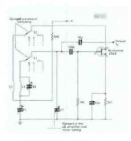
Fig. 2: The I.o. of a four band receiver based on an n-junction f.e.t. The tuned circuit and feedback of only one band is shown. The other three are similar except for component values. This v.f.o. is tuned over the selected band by C1.
