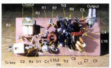
inductance value for L1 is 6µH and this resonates on 7.030MHz (the QRP Calling Frequency) with a capacitor of about 85pF. I used a trimmer I found in the junk box.
