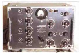
Fig. 1: The TA-12 transmitter, the four oscillators are situated down the left side, with the p.a. controls on the right and band changing controls in the centre (see text).
