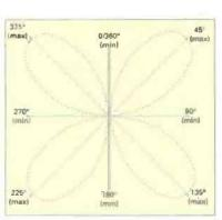
Fig. 2: Making an antenna a fullwavelength long gives four natrow lobes of maximum radiation and four distinct null-points, two of which occur at what was the maximum radiation direction of the halfwavelength antenna.
