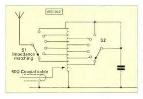
Fig. 5: A slight modification the the a.t.u. of Fig. 4, can sometimes improve the range covered,
