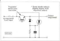
Fig. 4: A 'bare-bones' overvoltage protection circuit (see text).
