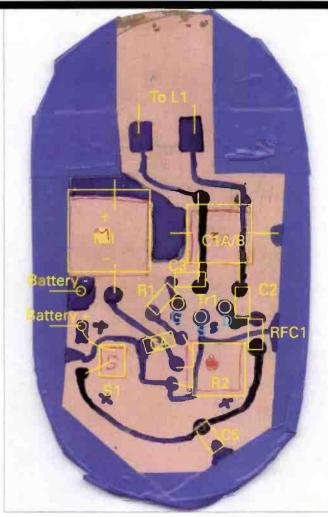
Fig. 4: The p.c.b. prepared and 'masked' with pvc tape ready for etching. The positions of switch, meter and potentiometer holes: are also marked (these should be done prior to masking and marking out).
