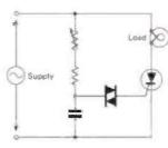
Fig. 3: The bare circuit details of a light dimmer circuit (see text).
