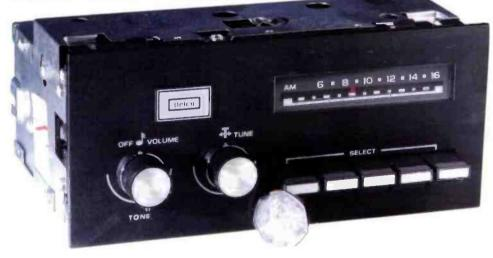
Fig. 1: The unusual 'Delco' (Made in Mexico for the American market) car radio which can be used as a 'tuneable intermediate frequency', photographed together with a 50p piece for size comparison. Looking almost like a miniature 'communications' receiver the radio is both sensitive and selective bearing in mind its original purpose.
