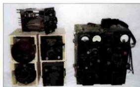
Fig. 3: The T1083 transmitter with associated coils (see text).
