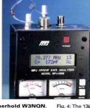
Fig. 4: The 13Ω reactive impedance of Fig. 3, might be a 172pF capacitor...
