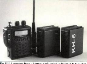
The KH-6 operates from a battery pack which is designed to take dry cell or NiCad type batteries. Also shown here is the sealed NiCad battery pack which is available as a optional extra (see text).
