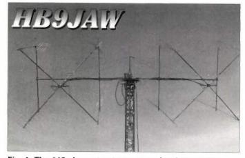
Fig. 1: The 448-element antenna array for the 144MHz band at the QTH of of Michel Winiger HB9JAW.
