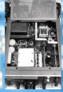
Fig. 4: Inside view of the T-599S transmitter. The p.a. stage is on the top right within the screened compartment, and the v.f.o. on the bottom left. Linking between the variable capacitor control shafts and the capacitors is by substantial 'non slip' chain drives!
