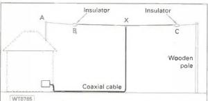
Fig. 1: This form of dipole is quite effective at h.f. and should work on all bands.
