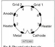
Fig. 5: The octal valve base pin numbering with the pinout details for the 6V6GT and the 6L6GT valves
