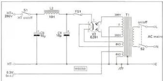
Fig. 2: This is a suitable p.s.u. to power the transmitter up to about 10W input power.
