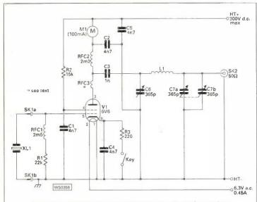
Fig. 1: The circuit for the single valve crystal controlled transmitter.
