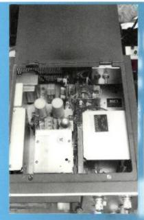
Fig. 3: Photograph illustrating the inside cabinet view of the JR-599 receiver. he built-in 144MHz converter can be seen at the top centre right, with space for the optional 50MHz converter alongside (see text).
