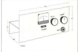
Fig. 3: The type and size of chassis used by Richard for his prototype.
