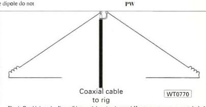
Fig. 6: Combining a loading coil into each leg of an inverted-V antenna can save a great deal of space for lower h.f. band antenna users.
