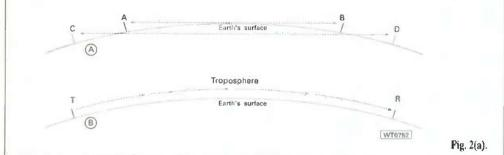
Fig. 2(a): The geometric horizon path AB and the radio horizon distance CD, where the wave follows the curved path of the earth owing to tropospheric refraction (shown at b).
