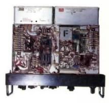
Again...the GR-345 is not really 'standing on it head'! This photograph shows the various unit interconnections and how small gold-plated other antennas or tuners to be plug and sockets route the r.f. signal through the various units.
