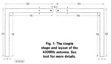
sections was drawn accurately and the shape then cut out. Scissors, or a straight edge and a sharp knife may be
