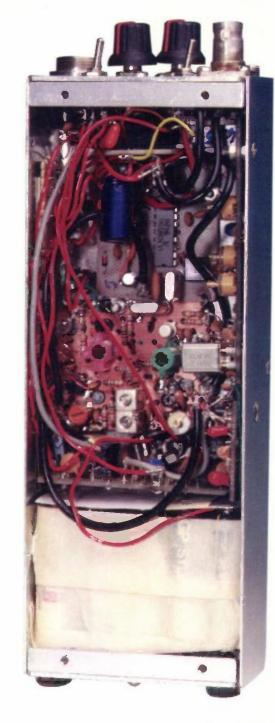
poor temperature dependent squelch control. Selectivity is provided by FL101, which is (typically) of 15kHz bandwidth.
