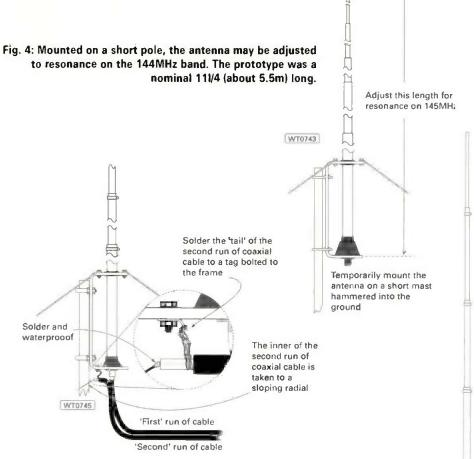
Fig. 5: A little more detail of how the second coaxial cable is attached. The connection within the dotted circle should be completely waterproofed with a bath sealant or similar.
