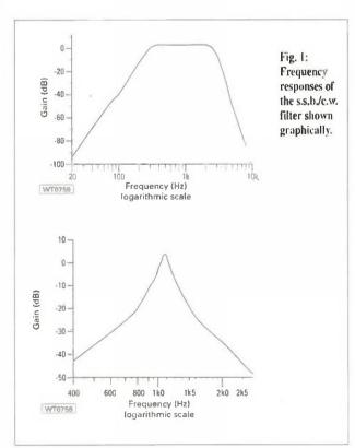
The filtering (or processing) will help to maximise the signal to noise ratio and hence intelligibility of the audio signal. With this in mind, I eventually decided to use four order of active high-pass filtering and twelth order of active low-pass filtering offering ultimate rejection rates of 24dB per octave and 72dB per octave respectively.
