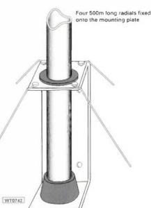
Now, take a length of  $50\Omega$  coaxial cable with a PL259 connector either end. Mount the fully extended antenna on a temporary pole. I found that a short alloy pole about a metre long hammered into the ground worked quite well, but mount the antenna as you can manage. Now you need to find the radiator length that gives the lowest s.w.r. on 144MHz (as shown in Fig. 4).
