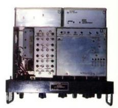
No it's not up-side down! It's easier to illustrate the various sub-units of the GR-345 this way and you can see the extensive screening used in the design.
