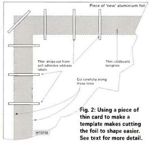
used to do this. Only one piece of card is required for it can be turned over to give its mirror image.
