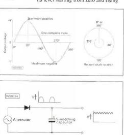
to a maximum positive before returning through zero to negative produces an annoying buzz. That's no good for us...so it has to be 'converted' or changed to a form that can be used and this is done by a device known as a rectifier.
