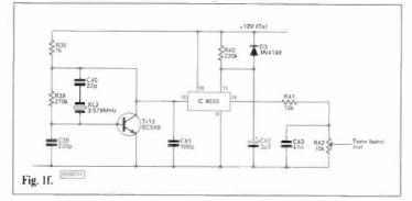
burst, produced by the circuit of Fig If is provided by a 3.579MHz crystal oscillator Tr12 and divided by 2048 using a MC4020 binary divider.
