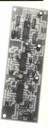
incoming audio from the receiver at line level is fed to C1, which acts as a d.c. 'blocking' capacitor and then to IC1, a quad operational amplifier.
