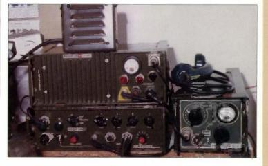
The Redifon GR-345 connected to the GA-480 amplifier and the ACU9 antenna tuning unit. (The loudspeaker on top has been borrowed from the GRC-9 radio).
