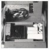
Fig. 4: The Mark 123 spares box showing wire antenna, spare valves and antenna insulators. Below is the 12V p.s.u. with leads. The device (top right) is the capacitor reforming tool (see text). an adapter for connecting the set to an external power source.
