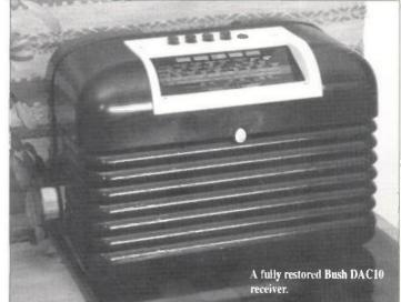
A rough estimate of a set's age. without looking inside, can be gauged by reading the station names on the dial. The 'Light Programme' was introduced in 1945 and the 'Third Programme' in 1946. However, bear in mind that pre-war dials were used by a few manufacturers for some time afterwards.
