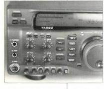
The left-hand side of the FT-920's front panel. The outer 'collar' control mounted directly behind the main tuning knob operates the 'Shuttle Jog' tuning control (see text).
