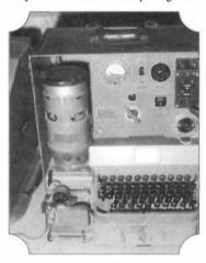
Fig. 2: The German Hellschreiher machine, showing the keyboard. The motor on the left forms part of the image scanning system.
