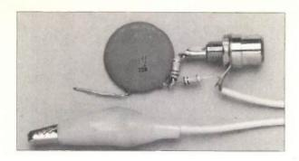
R6/R7, allows a low level signal from the oscillator to be used in testing audio circuits. The circuit is a basic resistive divider and values can be calculated for a desired output.
