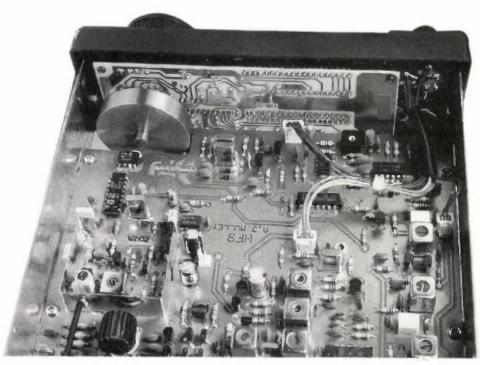
The smooth tuning action on the HF-3 is aided by a relatively large loaded flywheel, seen here mounted on the top left of the tuning sub-assembly panel.
