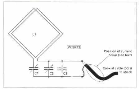
Fig. 1: The circuit of the 'Pile-Oop' antenna. Capacitor C2 is a 150pF variable, and C2 is a 500 + 500pF variable type. For details of C3 and the balun, see text.
