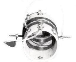
Fig. 4: Looking into the variometer unit. The rotor coil is at right angles (nil coupling) to the stator.
