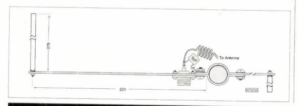
Fig. 3: Looking down on the 'ground' plane.
