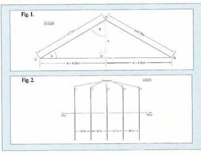
If, due to difficulties you cannot secure varying sizes of element to the woodwork, then I have a trick to help you out. Cut the total length of the reflector and directors all to be about 0.5m shorter than the calculations indicates
