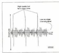
Fig. 1: A typical speech waveform.
