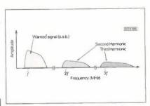
Fig. 3b: Clipping at r.f. showing the position of harmonics.
