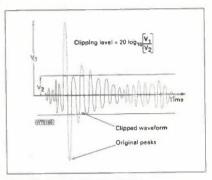
Fig. 2: Action of clipping a signal.
