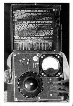
Fig. 2: The 'Aerial Coupling Equipment 'C' (For Wireless Set No.11). This unit employs a variometer and is housed in a wooden case (see text).
