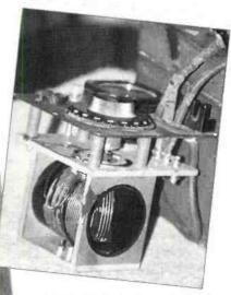
Fig. 5: The second set of wiping contacts can be seen in this photograph of the variometer, with the rotating coil (inside the fixed coil) clearly visible.
