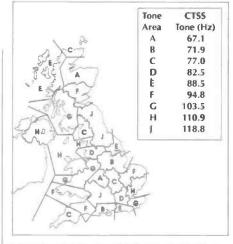
The plan to be used when a repeater uses CTCSS access.
