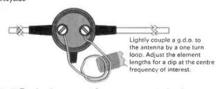
Fig. 2: To check resonant frequency, use a simple one or one and a half turn loop to couple a g.d.o. to the antenna.
