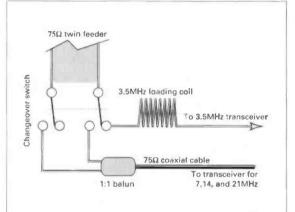
Fig. 2: Details showing feeding arrangement for 3.5MHz using loading coil and the 1:1 balun (see text) used for the 7, 14 and 21MHz bands. The 'end fed' input to the loading coil for 3.5MHz is via a crocodile clip or wander plug. Input from the transmitter to the balun is via coaxial cable, with termination to suit. The 28MHz antenna connection (using a retuned 27MHz vertical) at G3EAY's station is via a separate coaxial cable and PL259 plug.
