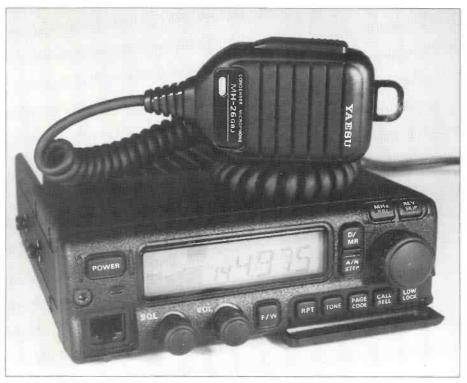
The Yaesu FT-2500M mobile transceiver.
