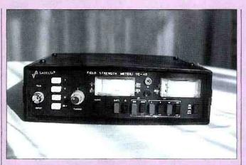
Fig. 1: Designed originally for domestic v.h.f. radio and TV signal strength metering, this f.s.m. from Sadelta is nonetheless very useful for amateur frequencies.
