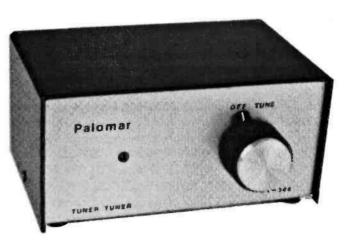
The Tuner-Tuner is a particularly neat device that connects between the transceiver and the a.t.u. The object being to enable the optimum a.t.u. settings to be found without having to transmit a carrier.
