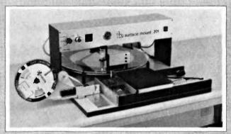
Fig. 2c. A fully manual 'pick & place' machine.
