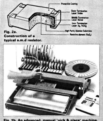
Fig. 2b. An advanced, manual 'pick & place' machine.
