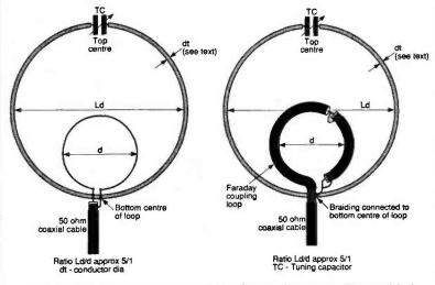
Fig. 2.8: Two methods (a and b) of coupling a small tuned h.f. bands loop antenna 5.34m circumference at frequencies between 3.5 and 28MHz in steps of 3.5MHz. See text for more details.
