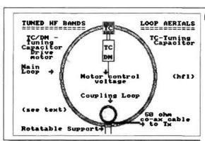
Fig. 2.4. Whilst the circumference for operation on three or four amateur h.f. bands may be physically constant, it does, in reality, vary inversely to the wavelength of the frequency in use. On the other hand the loop must be large enough to maintain an acceptable degree of efficiency, to minimise the 'loss factor' for each frequency band. This is shown more graphically in Fig. 2.5.
