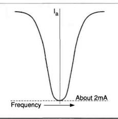
Fig. 5.3: The unloaded anode current as the frequency is swung about the resonance point of the circuit. This shows a distinct fall of  $\mathbf{i}_{\mathbf{i}}$  to about 2mA at resonance,  $\mathbf{R}_{\mathbf{b}}$  is about 125k $\Omega$ .
