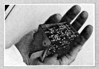
Fig. 13. G4ZQK's s.m.d. transceiver.
