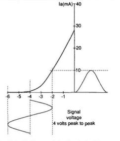
Fig. 5.4: At the new bias level of -4V showing the 'peakiness' of the anode current.
