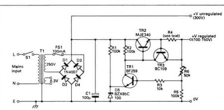
Fig. 1: The circuit diagram of the regulator, note the simplicity, the p.s.u. has only one capacitor.
