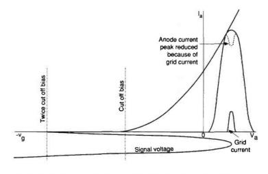
Fig. 5.6; Rather more drive, taking the valve into grid current, and the subsequent slight 'flattening' of the anode current peak.
