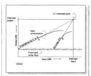
Fig. 6: A plot expressing the r.f. intercept point, which can be referred either to the input or output signal level. This is fully explained in the text.
