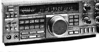
The R-5000 from Kenwood 100kHz-30MHz. SSB/AM/CW/FM/FSK
