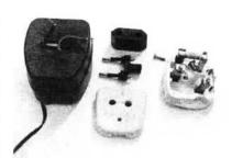
Power pack with original pin assembly removed
