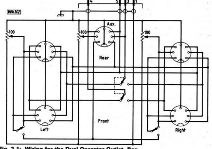
Fig. 2.1: Wiring for the Dual Operator Outlet Box
