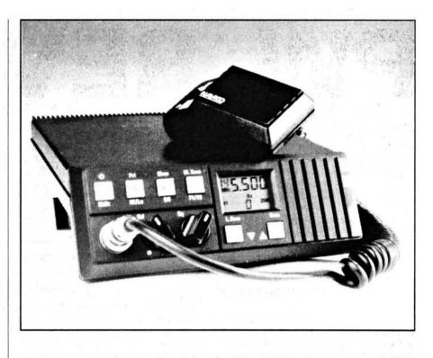
when you press the p.t.t., there is a carrier present, the tone burst is disabled, if however there was no carrier present, the tone burst circuit sends out a 400ms burst of 1750Hz to access the repeater. The idea is so simple I can't imagine why everyone isn't doing it, so full marks to Navico for some smart thinking!
