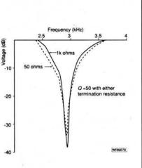
Centre Fig. 5: Rejection mode filter characteristics. Centre frequency 2.95kHz
