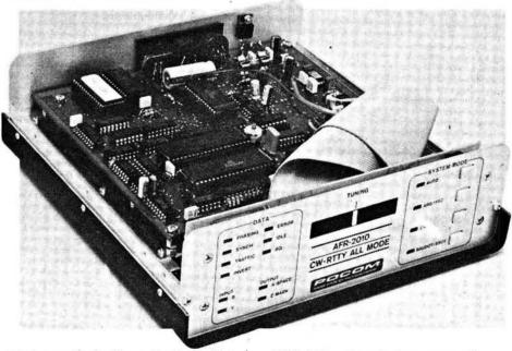
narrow vertical oblong. In the initial stage there is just one vertical l.e.d. alight in the centre, but as soon as a station is tuned in, or even as soon as any input is received, the rest of the l.e.d.s light up in a random fashion. As one tunes over the frequency and passes various types of transmission the tuning bar alters in brilliance and length. I will describe the appearance of the tuning bar for various types of signal later.
