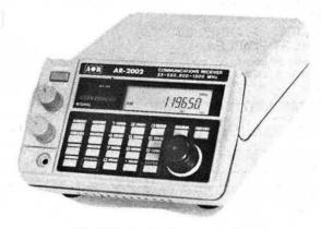
Frequency range of the AR2002 is from 25 to 550 and from 800 to 1300 MHz. Modes of operation are wide band FM, narrow band FM and AM. The receiver has 20 memories, memory scan and a search mode which checks frequencies between user designated limits.
