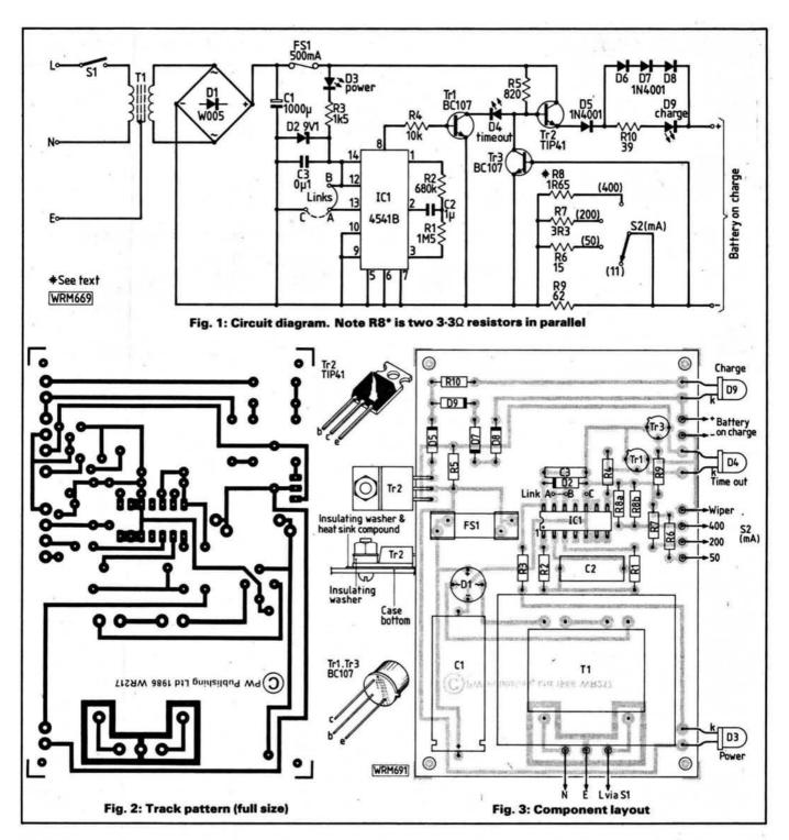
counting action starts at switch on. When the count is complete, 14 hours later, the output on IC1 pin 8 goes positive, switching on Tr1. At this point Tr1 diverts the base current from Tr2 through D4, to 0 volts, thus turning off the charge current and illuminating the TIME OUT l.e.d. The diode D5 prevents the l.e.d. D9 and the emitter of Tr2 being subjected to reverse voltage from the batteries when Tr2 turns off at the end of the charging cycle.
