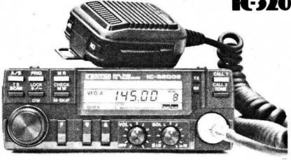
If you are a newly licensed or just undecided about which band to first operate, then the ICOM IC-3200E is just the answer. This is a dual-band (144-146/430-440MHz) F.M. transceiver ideally suited for the mobile operator. The IC-3200E has a built in duplexer and can operate on one antenna for both VHF and UHF, and with 25 watts of output power on both bands (the low power can be adjusted from 1 to 10 watts) you can never be far from a contact whether simplex or 2m/70cm repeater.
