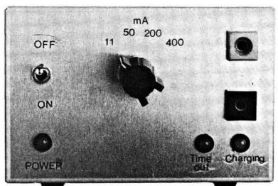
Front panel of completed NiCad charger.
