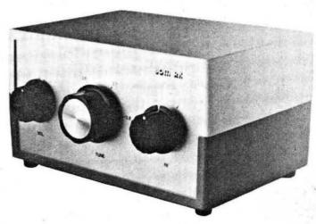
This is how we boxed the C.M. Howes receiver, a diecast box inside a Verobox
