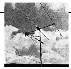
Fig. 2.4: Photograph of the prototype 50MHz 3-element beam. The item beneath the antenna is a wind direction indicator
