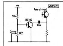
Fig. 1: Power output control on the pre-driver stage
