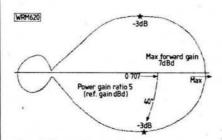
Fig. 2.6: Polar radiation pattern of the 3-element beam in horizontal mode
