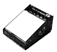
The CDA-1 is housed in a strong metal cabinet with a sloping front panel, and all metal parts are earthed the meet the most stringent safety regulations. The unit incorporates fuse protection and an a.c. mains switch with a built-in pilot light.
