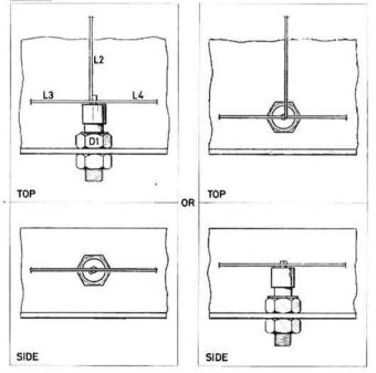
Fig. 5.7: The physical arrangement of L2/3/4 should minimise coupling; the above layouts work well
