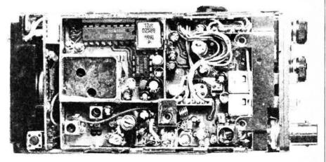
The screened r.f. deck of the FT-209RH. The c.p.u.s. are located on a separate p.c.b. mounted behind the keypad
