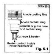
needed. One side of the heater is joined to the cathode so the heater winding must not be earthed. Arrangements are needed to feed the heater through suitable r.f. chokes because the cathode is "live" at r.f.
