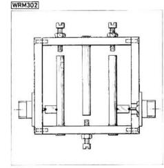
A cross-section through an interdigital bandpass filter. The tuned  $\lambda/4$  "finger" elements provide good harmonic rejection
