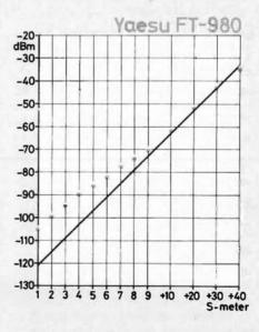
S-meter checks at 14.1MHz. The solid line is the IARU recommended scale; the dots show the actual input level required to produce the various readings
