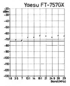
Variation of S-meter sensitivity with frequency. Again, the solid line is the IARU recommendation; the dots the actual input needed for an S9 deflection on each band
