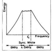
Fig. 3.1: Energy distribution of a simple grey scale
