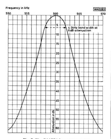
Fig. 5: The R1155 i.f. response curve
