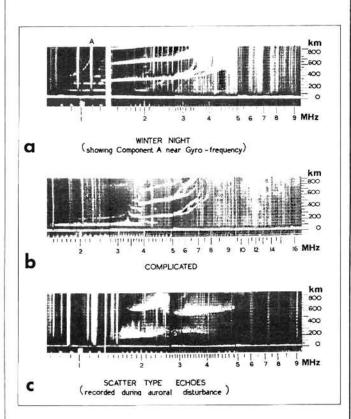
Fig. 4.3: lonograms showing other aspects of ionospheric sounding as explained in text
