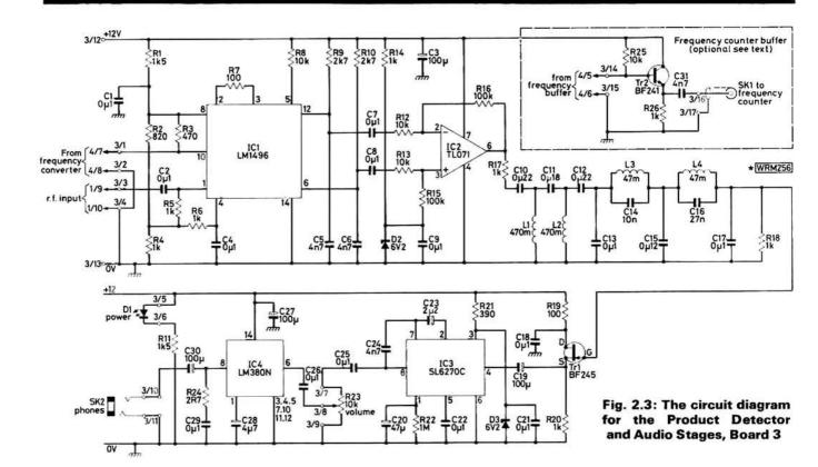
results in this application. As well as giving a high maximum voltage gain (52dB), the output of the i.c. remains essentially constant for a 60dB input voltage range. A full description of this i.c. is not given here and further details can be obtained from the Plessey data. The attack and delay times and frequency response of the circuit is set by the external components 3C20, 3R22, 3C23 and 3C24. The maximum operating voltage is 10V and so a supply rail is generated
