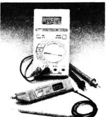
The versatile DM73 is ideal for voltage and resistance measurements in hard-to-reach locations. It has four a.c and d.c. voltage ranges from 2V to 500V, four resistance ranges from  $2k\Omega$ to  $2M\Omega$ , plus a buzzer for continuity. testing and circuit tracing. Also, a "display-hold" button facilitates measurements to be held on the display after the probes have been removed from the circuit. The DM73 is priced at £39.75.
