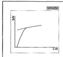
Fig. 3.3: The detection threshold characteristic of an f.m. system
