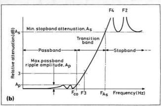
Fig. 5.1: Circuit diagram and attenuation response of 5-branch Cauer lowpass filter. Tune C2/L2 to F2, C4/L4 to F4
