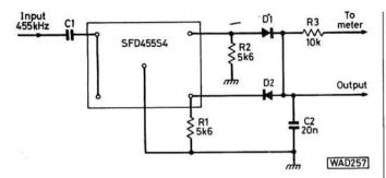
Fig. 6: Ceramic ratio detector using the SFD 455S4 (Toko/Yaesu FT 227)
