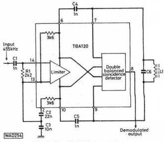
Fig. 3: The TBA120 demodulator
