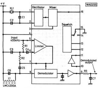
Fig. 4: The MC3357/MP5071 demodulator system.
