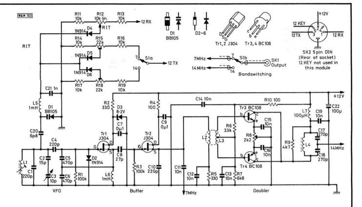
Fig. 2.1: Circuit diagram of Module 2, the VFO/Doubler
