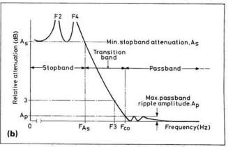
Fig. 5.2: Circuit diagram and attenuation response of 5-branch Cauer highpass filter. Tune C2/L2 to F2, C4/L4 to F4
