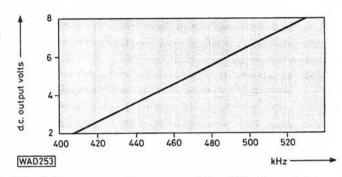
Fig. 2: Linear operating range of the 4046 demodulator
