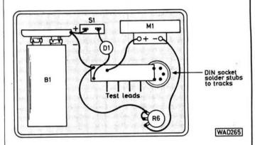
Carry out the same checks using an f.e.t. or dual-gate m.o.s.f.e.t.—the fourth terminal marked Gate 2 on Fig. 1 provides a fixed d.c. bias. If a transistor under test does not produce any output once the unit is functioning properly it is either unserviceable or has a low  $f_t$  and therefore should be tested on a d.c. transistor tester as described on page 37.
