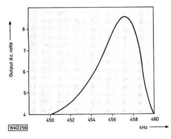
Fig. 7: Response of the TBA120 with 8008 ceramic resonator
