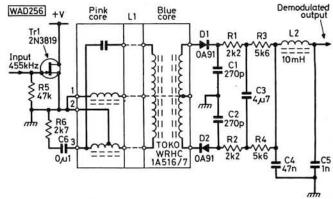
Fig. 5: Discrete component ratio detector
