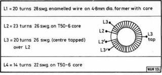
Fig. 2.2: Coil winding details for the VFO/Doubler module
