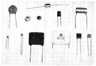
Capacitors should be chosen with a working voltage well in excess of what they will have to withstand
