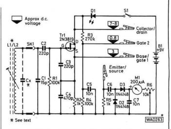
Fig. 1: Circuit diagram of the simple r.f. transistor tester
