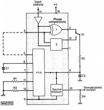
Fig. 1: Block diagram of the 4046 p.l.l.
