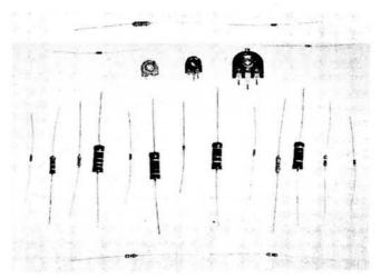
Different types of resistors and potentiometers with between 0-125 and 2 watts power ratings
