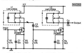
Fig. 9: Circuit diagram of a 455kHz i.f. amplifier
