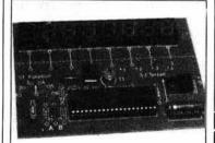
10MHz DEM CRYSTAL CALIBRATOR Crystal reference calibrator for alignment of receivers, outputs at 4, 2, 1MHZ, 100, 50 AND 10KHz 41-00801 4.32 CB NOISE SQUELCH Improves the mute performance of the majority of CB rigs 41-01605
