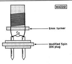
Fig. 3: (Above) Details of the plug-in coils. Fig. 4: (Below) Suggested layout of the unit in a plastics box
