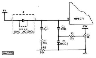
Fig. 8: A tunable 455kHz demodulator using the MP5071
