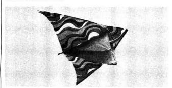
The Twin Keeled Delta kite which is suitable for antenna support is available from Cochranes of Oxford Ltd., Leafield, Oxford OX8 5NT, Tel. 099 387 641
