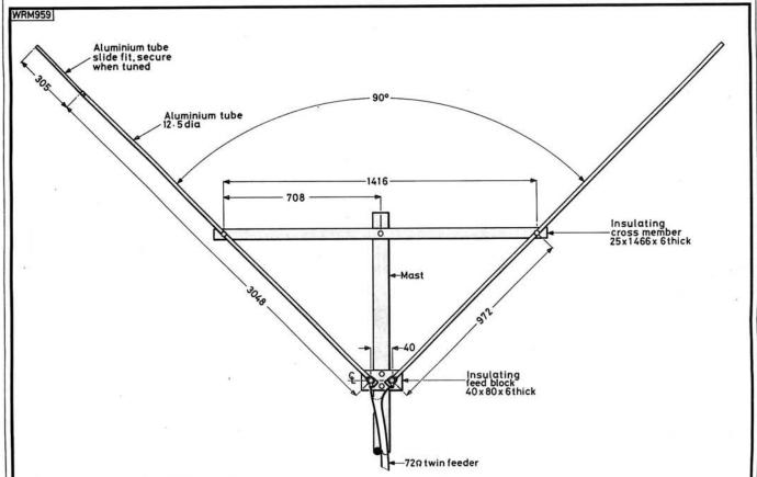
Fig. 1: Constructional details of the Vertical V antenna for 21MHz. Both radiating elements are provided with length adjustment and for best results a 1:1 balun should be fitted at the feedpoint when using 50 ohm coaxial cable. Note that this drawing is not to scale
