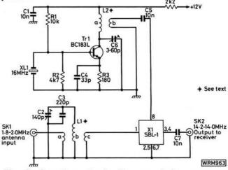
Fig. 2: Complete circuit diagram of the converter which will provide 1-8MHz band coverage when used in conjunction with a 14MHz receiver
