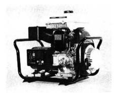
A Calor gas conversion kit is being produced, which will cost around £45 and will offer the advantages of cleaner burning, less dangerous exhaust fumes, quieter running, plus a 26lb bottle of gas will run the generator for approximately 26 hours.
