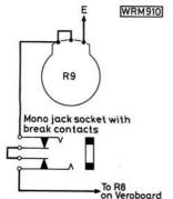
WRM910 Fig. 4: The modification needed to provide a Morse practice facility. The jack socket which should be a mono type, can be located on the rear panel of the filter housing
