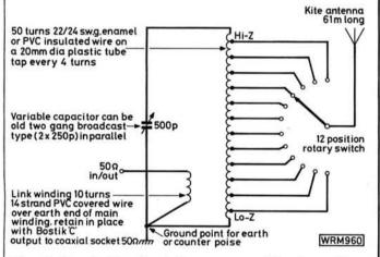
Fig. 2: Circuit details of the a.t.u. used by the author for operation on the 1-8MHz band
