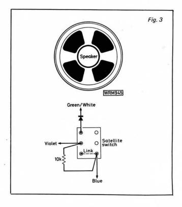
Next, unsolder the green/white wire from the topmost pin and solder a diode (1N914) to that pin. Then solder the green/white wire to the other end of this new diode. Now, whenever you are listening to a repeater, pushing the toneburst button on the microphone will cause the receiver to switch to the input.
