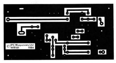
Fig. 3: Full size p.c.b. and component placement details. Pin 2 of the mixer X1 is located beneath the letter M of the part identification
