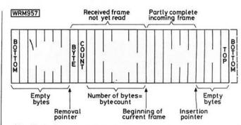
Fig. 2.6: A typical data buffer, showing pointers, and order of placement data. The buffer shown is the packet input buffer, and is similar to the other buffers
