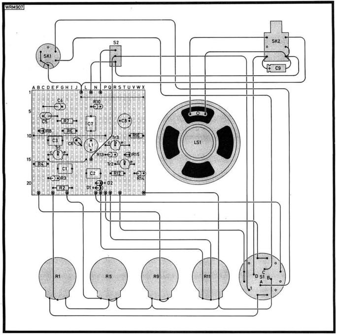
Fig. 2: Component placement and interconnection details. Veroboard track breaks occur at M7, M12, O12, E19 and N18
