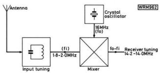
Fig. 1: Block schematic of the PW Dart 1-8MHz receive converter
