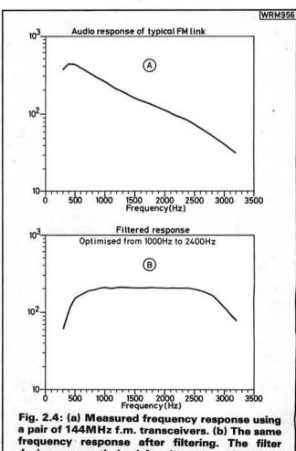
design was optimised for the range 1000Hz to 2400Hz
