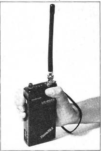
The  $50\Omega$  flexible antenna plugs into a BNC socket on the top panel where the volume/off switch, squelch and frequency selector switches are also located. Frequency selection is achieved with "thumb-wheel" switches and depending on the size of your fingers can be easy or difficult to operate.
