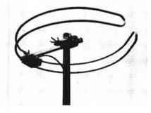
Gain is claimed to be between -2 and -4dBd and the folded element is constructed of 3 in diameter seamless aluminium tube.
