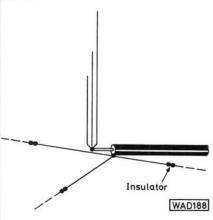
Fig. 2: If at all possible horizontal wires should be added as shown here, all soldered together and to the outer shield of the coaxial cable. The wires are the same length as those in the vertical elements, one for each band, but two or more per band are highly desirable
