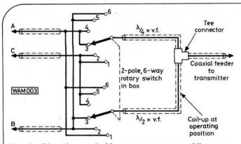
Fig. 3: Direction switching arrangements. Allowance must be made for cable velocity factor (v.f.)
