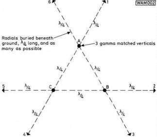
Fig. 2: Plan view of the system. The vertical elements are spaced  $\lambda/4$  apart at the operating frequency
