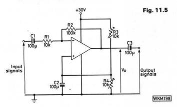
Capacitors C1 and C3 are d.c. blocks which prevent the d.c. conditions of other stages from upsetting the critical d.c. conditions of the op. amp. circuit. As far as signals are concerned C2 earths the "+" input but allows the correct d.c. potential to exist there.
