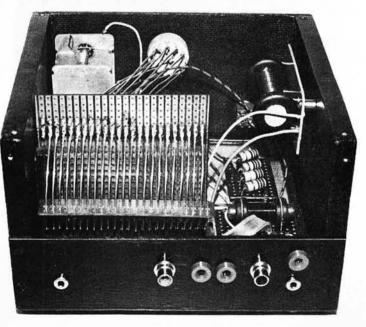
Cardboard discs are glued behind the knobs and marked by Letraset or similar system. The discs used were obtained from the local stationers in the form of "conference badges". The centres were removed by perforating them with the aid of a domestic sewing machine.
