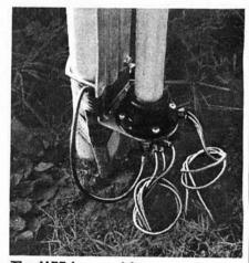
The HF5 base, with connections to five buried radials for improved soil conductivity
