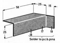
Fig. 2.3: The folded tinplate p.c.b. screen
