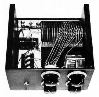
and C2 in conjunction with each other. C1 in the prototype was of the type used in valve receivers, which can often be obtained cheaply as surplus components. Neither value is very critical. If bought new Jackson type OO twin-gang 365pF would be suitable for C1 and type O single-gang 365pF for C2.
