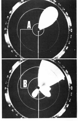
Fig. 3.5 (A): Prototype radiation pattern at midfrequency (from horizontally polarised wave). Fig. 3.5 (B): Amplified rear section showing low level back lobes
