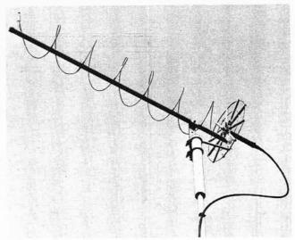
icle we dealt with the basic enna and its relatively wide Fig. 3.1: The author's prototype six turn helical antenna
