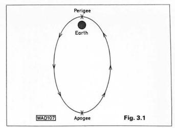
Africa, Asia and North America. Further, due to the nature of an elliptical orbit it will appear to be almost stationary (i.e. in the same part of the sky) for about 3 hours either side of apogee, a total of 6 hours per orbit.
