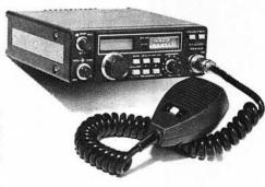
tion, priority channel, scanning and priority checking and memory shift operation. A red l.e.d. indicates that the rig is in transmit mode while a matching green l.e.d. shows that the squelch is open. An analogue meter indicates signal strength on receive and r.f. output power during transmit. Manual tuning is carried out by rotating the large knob below the digital display panel.
