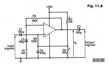
As before C1 and C3 are d.c. blocks. Capacitor C2 allows the negative feedback to the "-" input to be due to signals only. The +15V bias is decoupled to the "+" input via C4, and R5 allows input signals to be developed across it, being connected between the "+" input and earth as far as signals are concerned.
