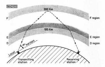
Fig. 1: Outline of the ionosphere. Region F, which reflects h.f. and is formed by uv radiation from 100 to 1000Å, contains the bulk of free ionisation. The E region reflects m.f. at night (when the D region does not absorb) and is produced by radiation from 10 to 100Å. Region D is an ill-defined layer which causes radio-wave absorption and is produced by uv wavelengths greater than 1000Å during quiet solar conditions or by 1 to 10Å X-rays from solar flares
