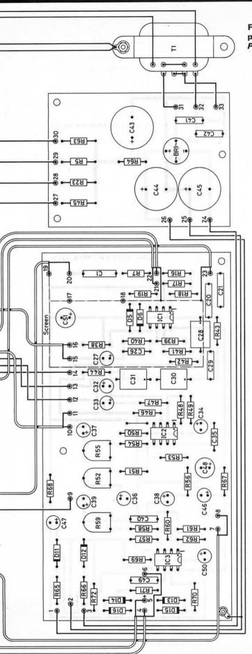
Fig. 2.1: Interconnecting wiring diagram, full-size p.c.b. track patterns and general layout details of the PW Durley. The rear view of the front panel is shown two-thirds full size
