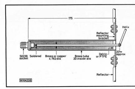
Fig. 3.3: Constructional details of the  $\lambda/4$  matching transformer which has an impedance of approximately 86 ohms to provide a match between the 50 ohm coaxial feeder cable and the 140 ohm characteristic impedance of the helical antenna. The line impedance is derived from the formula:
