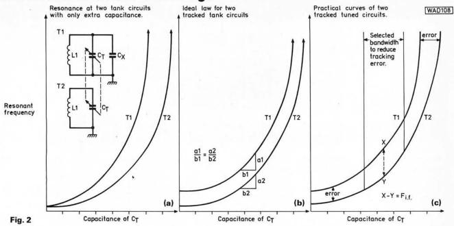
simply adjusting one factor defining the resonant frequency of the circuit, we will certainly not get the ideal curves we require. The ideal curves are shown in Fig. 2(b). Notice how the curves for each idealised network have the same gradient, and that all along the graph the following relationship will apply.
