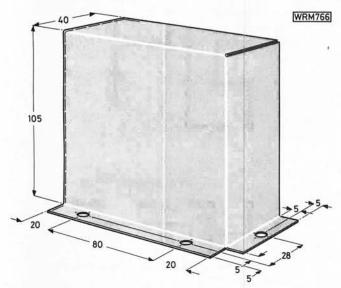
Fig. 2.2: Details of the 18 s.w.g. folded aluminium input section screen located over SK1, S1, 2 and 5
