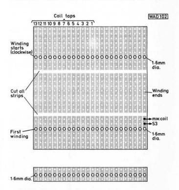
Fig. 2: Details of the 0-15in matrix Veroboard used to support the main coils
