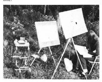
Fig. 6: A simple makeshift set-up for viewing projected solar images employs a pair of binoculars (only one monocular used), a shielding board and an imaging board. This apparatus was actually used to view a solar eclipse in 1976 high on top of a mountain in SE Australia. The author's wife records temperature and light values in the background. Eclipses historically helped identify the agencies responsible for producing the ionosphere
