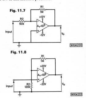
No. 1: Calculate the d.c. potentials at the "+" and "-" inputs and the value of Vo if the following d.c. inputs are applied to the circuits of (a) Fig. 11.7 and (b) Fig. 11.8.
