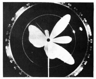
Fig. 3.6 (a): (left) Six turn helical antenna radiation pattern at mid-frequency from vertically polarised wave. Fig. 3.6 (b): (right) Break-up of uniform radiation pattern at extreme limit of frequency coverage
