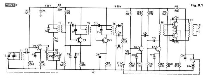
Transistors Tr6 and Tr7 voltages will be identical under no-signal conditions, since there is no resistance in T6 or T7 and the emitters are joined together.
