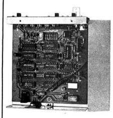
Accuracy, like that of the FC-841, was quite remarkable. The makers specify  $\pm 50$ p.p.m. from 0-40°C, and importers Holdings of Blackburn reckon  $\pm 3$ p.p.m. at room temperature. Checked against an ovened 1MHz standard over 24 hours in a room varying from 15° to 21°C, the readout varied by only 2Hz. The readout is not all that bright, and you'll need to find a shady corner, away from sunlight or a bench lamp.
