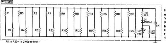
Fig. 2: Circuit of the 50 ohm dummy load. The Western Electronics PM2001 meter (above) handles 200W continuous r.f. power at frequencies up to 150MHz. It also indicates v.s.w.r.
