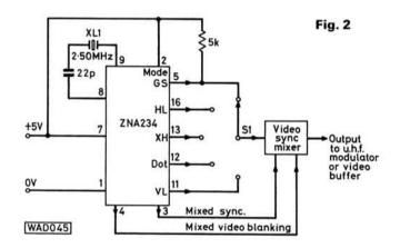
particular type of pattern required and feeds this signal either via a simple buffer stage to the receiver video circuit, or to a suitable modulator, producing a signal which can be fed into the TV antenna input.
