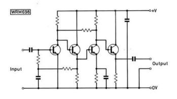
Fig. 1: Basic wideband gain-block
