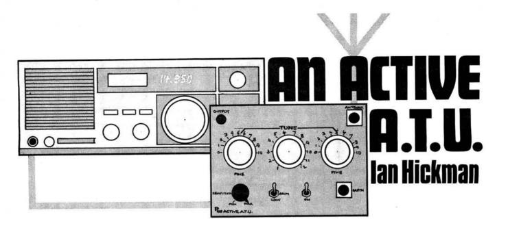
The unit described in this article is suitable for use over the approximate frequency range of 750kHz–25MHz, i.e. the greater part of both Medium and Short wavebands. A conventional antenna tuning unit (a.t.u.) enables almost any antenna, long or short, to be matched to a receiver, ensuring maximum transfer of r.f. energy from the antenna to the receiver's input stage.
