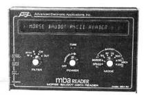
I.e.d. indicators. The THRESHOLD control on the reader is first adjusted so that both I.e.d.s are extinguished with no incoming signal. Then, the receiver tuning and audio level should be adjusted until both I.e.d.s flash in time with the signal for Morse, or so that one is continuously lit and the other flashes in time with the signal for RTTY modes.
