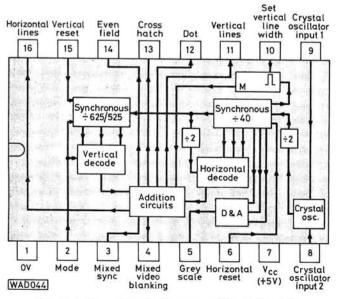
Fig. 1: Internal block diagram of the ZNA 234
