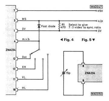
pin 12; it can be seen in Fig. 3 that the waveform at pin 12 is "high" only when the waveform at both pins 11 and 16 are also high.
