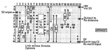
Fig. 4: Full-size layout details of the components of the a.t.u. The photograph shows the outline position of the Veroboard
