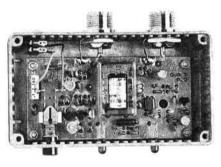
The review sample was tested on a rather ancient and "deaf" v.h.f. communications receiver, giving quite a worthwhile boost to performance, and also with an h.f. amateur bands transceiver. The extra gain was successful in lifting US f.m. repeaters around 29.6MHz out of the mush and turning them into readable signals. On the bench, gain was measured at 9dB with a ripple of less than 0.5dB up to just over 170MHz. At 190MHz gain was down by 0.5dB and at 200MHz by 1dB.
