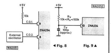
It should be noted that if pin 10 is not used, any stray external capacitance connected to this pin, such as a longish lead or the track on a p.c.b., will affect the circuit operation. Ferranti Electronics therefore recommend that if pin 10 is to be left open circuit, no connection at all should be made to it.
