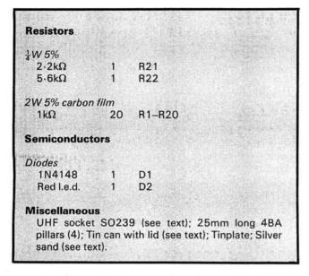
connected in parallel. Each resistor has a value of 1000 ohms so the total value for parallel connection is  $1000 \div 20 = 50$  ohms. The input is via an SO239 socket and the unit is equipped with an l.e.d. that indicates power present in the load. This will glow with a minimum power of 1 watt into the load but not exceed normal brilliance at high input power levels.
