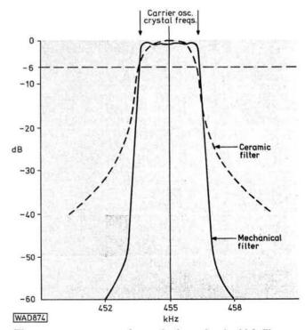
The response curve of a typical mechanical i.f. filter at 455kHz is shown above. Compare with that of a ceramic filter noting the difference in the bandwidth of the skirts. The placement of the frequencies of the carrier oscillator crystals is very critical if good results are to be obtained on s.s.b.
