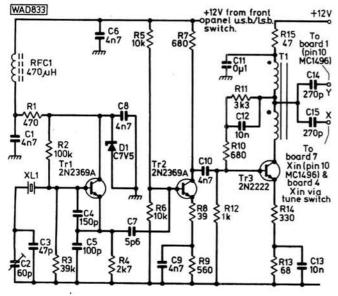
Fig. 6: Circuit diagram of Board 2
