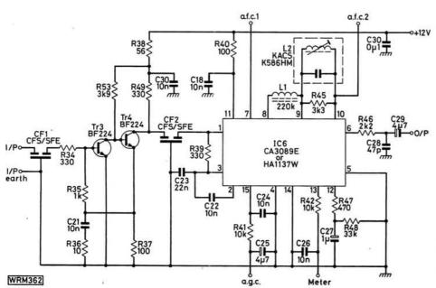
Fig. 5: The circuit diagram of the 10-7MHz i.f. unit. This is based on a circuit by Ambit International
