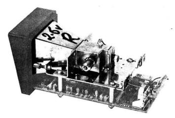
This burglar alarm, made by Wessex Alarms, is readily available on the surplus market. It can be used with the PW Exe system by retaining its horn antenna
