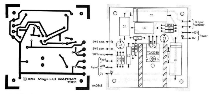
Fig. 4 (above): The copper track pattern for the p.c.b. shown full size. Fig. 5 (above right): The component placement drawing for the supplementary car audio amplifier printed circuit board
