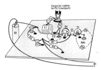
Fig. 2: The layout of the components is critical and this drawing should be followed for the best results. The picture on the right shows the completed prototype amplifier
