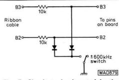
Fig. 7: Circuit to be inserted in the break for semi-reverse repeater mod
