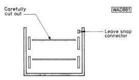
Fig. 1: One half of the battery pack BP4 with dry cell battery partitions to be removed
