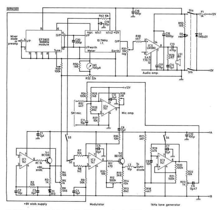
Fig. 4: The complete circuit diagram of the PW Exe transceiver. The 100MHz module is a high performance Band II tunerhead made by Ambit International. The 10-7MHz i.f. is shown in detail in Fig. 5
