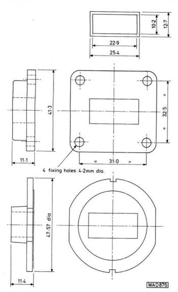
Fig. 3: Waveguide 16 flange details
