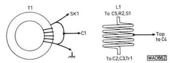
Fig. 3: T1 is a toroidal transformer consisting of 5 turns of 36 s.w.g. bifilar wound on a B64290 A36  $\times$  1 toroid. L1 is 5 turns 20 s.w.g. 6.4mm diameter tapped at  $2\frac{1}{4}$  turns
