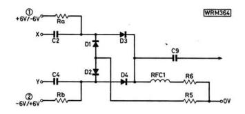
Fig. 10: Explanatory diode switching operation circuit
