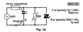
Unfortunately, its minimum impedance is limited by the need for a series resistor. This prevents the capacitor dumping its charge across the triac when the latter turns on. Such rapid discharging could easily exceed the di/dt rating of the triac. The resistor also prevents any spurious oscillation and ringing which can be readily precipitated by the step waveform of a transient, particularly when the circuit contains inductors.
