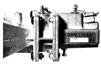
Plessey's GDHM 1 intruder alarm unit was used for most of the prototype PW Exe trials. This unit was also used for the PW Parkhurst burglar alarm and while proving to be very sensitive and stable, suffers from low r.f. output when re-tuned for amateur band
