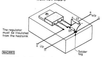
Fig. 3: Physical layout for the components in the battery compartment
