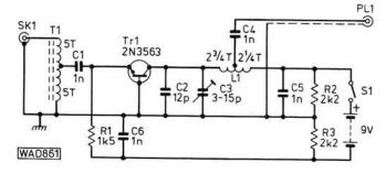
Fig. 1: The circuit diagram of the v.h.f. pre-amplifier
