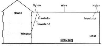
Fig. 1: The Inverted "L" Antenna
