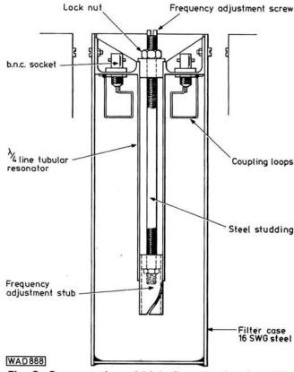
Fig. 2: Cross-section of high Q cavity developed by Roy Powers G8CKN. Internal faces are silver plated
