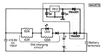
Fig. 4: Circuit diagram with components in the shaded area being additional
