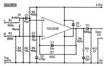
Fig. 2: The circuit diagram of the supplementary car audio amplifier
