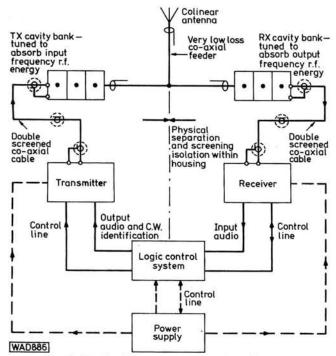
Fig. 1: Typical 2m repeater system diagram
