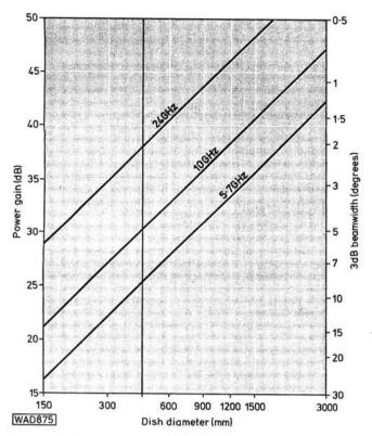
Fig. 6: This graph shows the effect of the diameter of a parabolic metal dish on its gain and bandwidth
