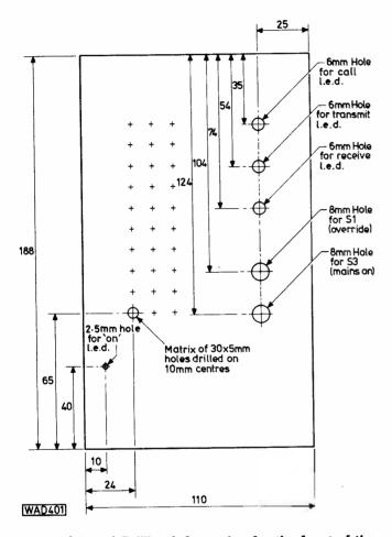
Fig. 4: (above) Drilling information for the front of the master unit. Fig. 5: (below) the details of the end of the master unit
