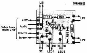
Fig. 6: Component placement and (top) the copper track pattern of the p.c.b. for the door unit shown full size
