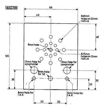
Fig. 3: Drilling information for the front door unit
