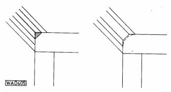
Fig. 2: (a) (left) marking for rounding edges; (b) (right) Initial planing of edge completed
