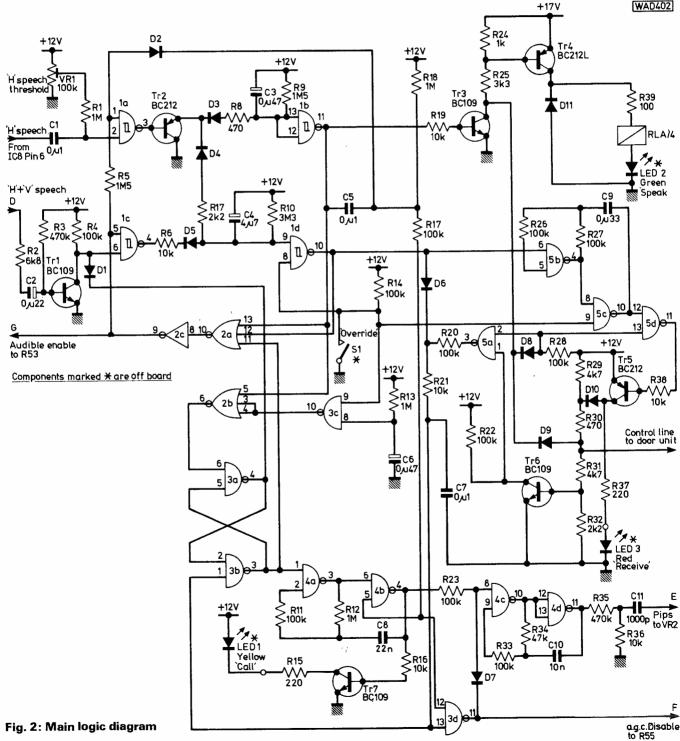
causes LED1 to illuminate. The potential across C8 is now reversed and it charges to the point where 4b pin 6 goes 'hi' again. The output of 4b reverts to 'lo' and Tr7 and LED1 switch off again. Capacitor C8 discharges until 4b pin 6 is 'lo' again, taking the output of 4b 'hi' and switching Tr7 and LED1 on again. The cycle will repeat for as long as the visitor continues to press S2—LED1 flashes and alternate 'hi' and 'lo' inputs are applied to pin 8 of gate 4c.
