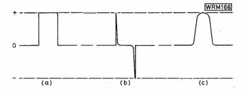
Fig. 2: The output of the high pass filter (b) and low pass filter (c) for a rectangular pulse input (a)
