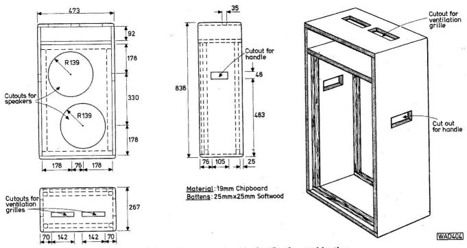
Fig. 1: Dimensions and assembly details of a combination amplifier/loudspeaker cabinet
