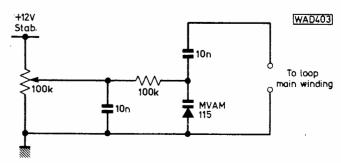
Fig. 1: A medium-wave loop tuning circuit using a varicap diode
