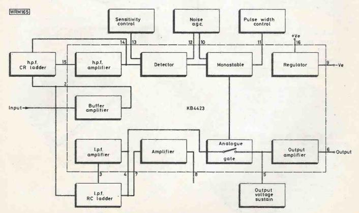
Fig. 1: General arrangement of the f.m. noise blanker based on the KB4423 i.c.
