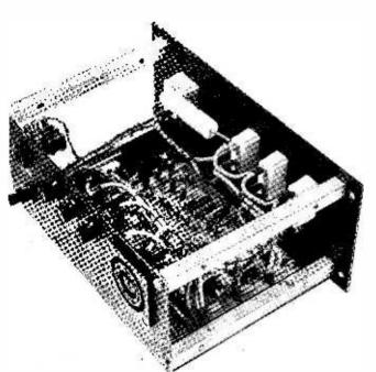
Chassis construction used in the PW "Soundlite"
