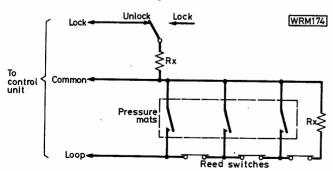
Fig. 3. A very basic 2-wire security circuit. Devices are shown in the "non-alarm" condition
