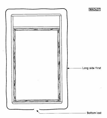
Fig. 3: Applying covering material to the cabinet
