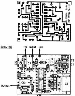
Fig. 4: Component layout and copper pattern of the p.c.b. (shown full size).
