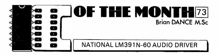
The design of high quality audio power amplifiers is quite complex, and poorly constructed circuits may develop distortion or even burn out if used in a warm room. To avoid the problems associated with the construction of a complete amplifier using discrete semiconductor devices, a complete audio hybrid module or integrated circuit power amplifier can be used.
