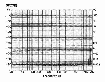
Fig. 5: CCIF intermodulation distortion produced by the Sony TA-N88 p.w.m. amplifier when delivering 38V peak composite signal across a load corresponding to a "difficult" loudspeaker of about 5 ohms modulus of impedance and 60 degrees phase-angle
