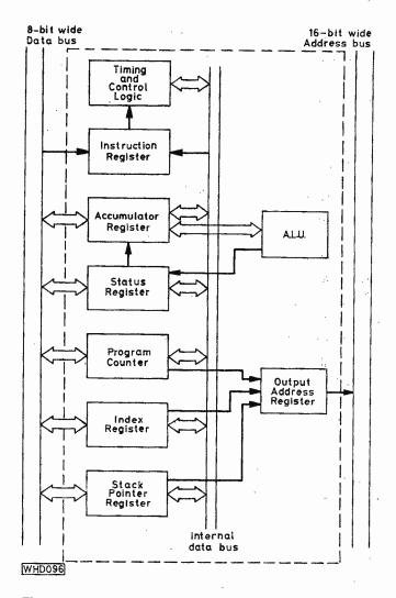
Fig. 82: Block diagram of a simple microprocessor chip
