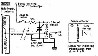
40 turns clockwise 40 turns anticlockwise on 7" ferrite rod (F11 or F14 material—preferably fluted)
