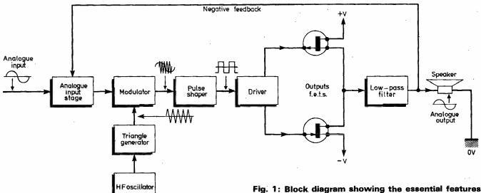
of the pulse chain. When there is no analogue input the pulse chain assumes a steady-state 50:50 mark/space ratio, which means that the tops of the pulses and the
