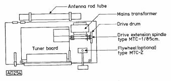
Fig. 11: Mechanical layout of the tuner
