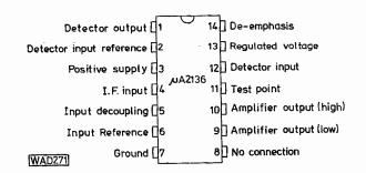
Fig. 8: The µA2136 connections
