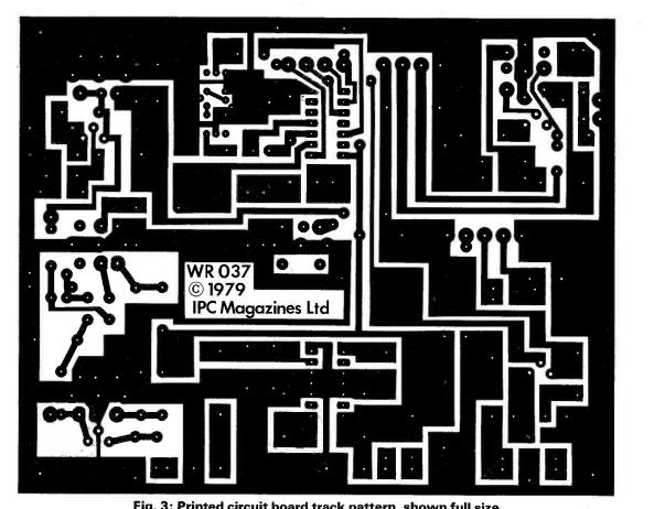
Fig. 3: Printed circuit board track pattern, shown full size
