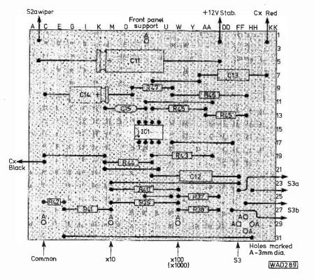
Fig. 1: The component layout of the add-on millifarad extender unit. 0.1 inch pitch Veroboard is used. The 741 op. amp. i.c. is shown as an 8 pin d.i.l. package but the alternative 14 pin d.i.l. package can also be used on the same board layout
