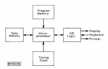
Fig. 83: Block diagram of a typical microcomputer system
