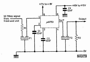
Fig. 7: A simple  $\mu$ A753 10.7MHz amplifier with ceramic filters
