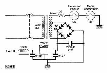
Fig. 12: Power supply arrangements
