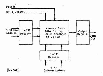
Fig. 78: Organistion of a typical 1024-bit (1K) memory
