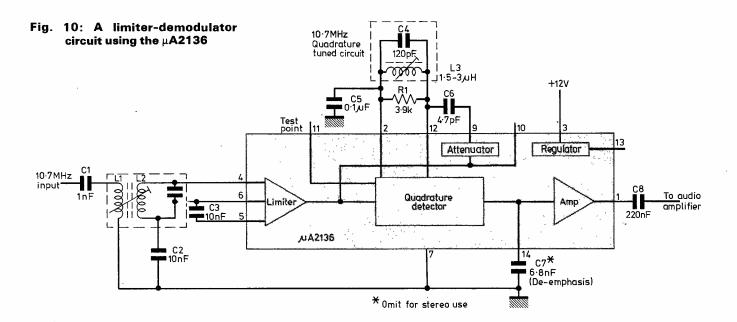
The output from the quadrature circuit is amplified and fed to pin 1. A de-emphasis capacitor should be connected from pin 14 to ground, the internal resistance of the device at pin 14 providing the required resistive component of the de-emphasis network.
