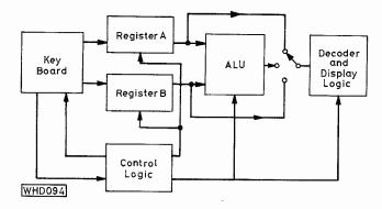
Fig. 81: Block diagram of a digital calculator
