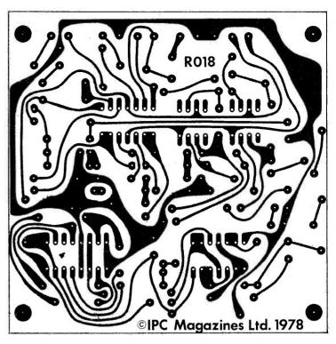
Fig. 2: Copper track layout (shown full size)
