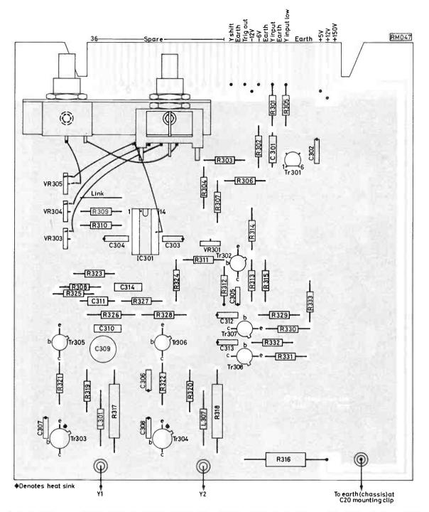
Fig. 3: The component layout of the Y amplifier board. Note that the components are mounted on the copper ground plain side of the board
