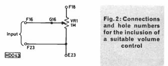
When you have "plugged" the components into your  $\mu$ DeC by their own leads (see Fig. 1) you should connect 6V to holes' Q1(+) Q23(-). The input is connected to holes F22 and E23. On test it was found that almost any microphone would work well and give a horrendously fuzzed voice output. Those tried included a cheap crystal insert, a commercial crystal microphone, a magnetic type (some 300 $\Omega$  impedance), and a small loudspeaker. Even small earpieces were tried and found to work.
