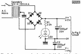
Fig. 3. A power supply circuit suitable for driving the Fig. 2 circuit
