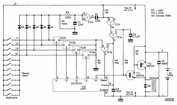
Fig. 2: Circuit diagram for the complete digital lock
