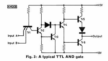
stops conducting if both emitter inputs are at 1. Transistors Tr5 and Tr6 form a "totem pole" output stage which gives a low output impedance and fast switching. For a 1 output Tr5 is "on" and Tr6 is "off" and vice versa for the 0 state. Thus the output is clamped to either 0V or +5V through one or other of the output transistors. The other transistors in the circuit provide the required drive signals for the output stage.
