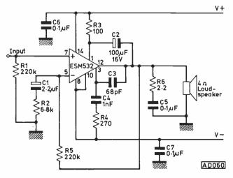
Fig. 2. A 20W amplifier circuit using balanced power supplies
