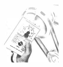
Graham and White's microprocessor-controlled tachometer.
