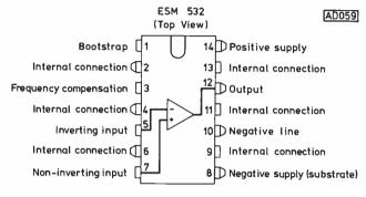
Fig. 1. The connections to the ESM 532
