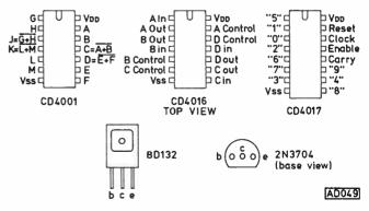
Connections to the integrated circuits and transistors
