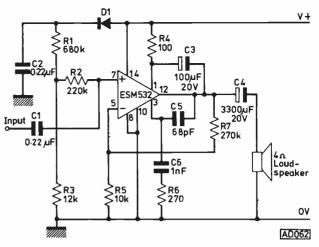
Fig. 4. A 20W amplifier using a single power supply
