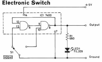
When testing JK flip-flops it is unsatisfactory to use an ordinary switch connected to the clock input. This electronic switch uses a 7400 i.c. in an 'anti-bounce' circuit, with an l.e.d. to indicate a high or low output.
