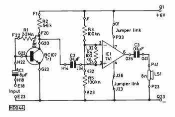
Fig. 1: Main circuit diagram including preamplifier
