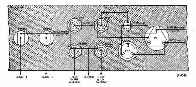
Fig. 8: Mains wiring and connections to the fuse-holders.
