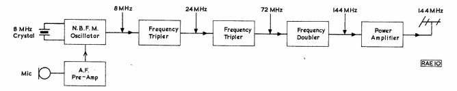
Fig. 61 : Block diagram of an n.b.f.m. transmitter.
