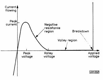
Fig. 2: Characteristic curve of the lambda circuit.
