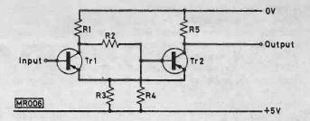
Fig. 3: The circuit of Fig. 2 modified to provide a greater "high" output drive capability.
