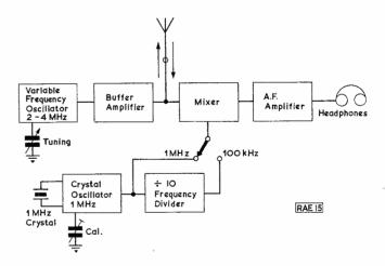
Fig. 66: Block diagram of a heterodyne frequency meter.
