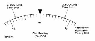
Fig. 67 : Interpolating between crystal calibration points.
