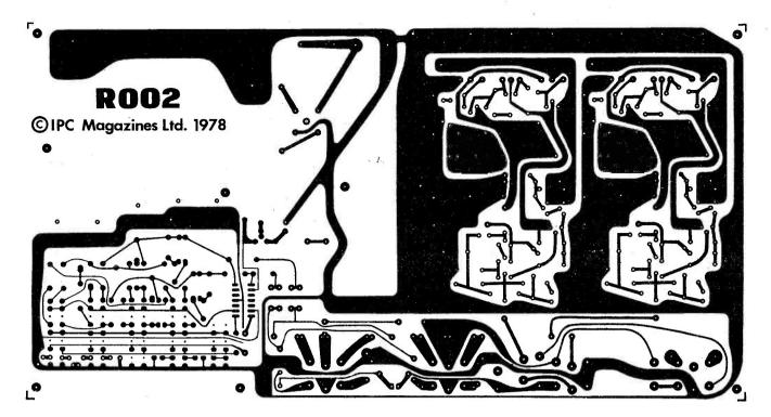
Fig. 4(b): Track pattern of the printed circuit board, shown half-scale. Full-size copies of this drawing will be available from the editorial address given at the front of the magazine, price 30p. Send a chequel postal order for 30p together with a large stamped self-addressed envelope. Ready-made boards will be available from the Readers PCB Service as usual. See their advertisement.
