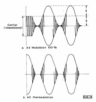
Fig. 70: Modulation patterns for an A3 signal. Note that in the overmodulated condition, flattening of the peaks will usually occur.
