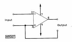
Fig. 1: The open-loop inverting amplifier circuit.
