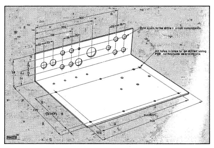
Fig. 5: Chassis dimensions and drilling details.
