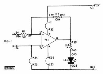
Fig. 3 : A practical inverting amplifier for you to make up.
