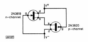
Fig. 1 : The basic lambda circuit configuration.
