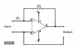
Fig. 2: The closed-loop inverting amplifier
