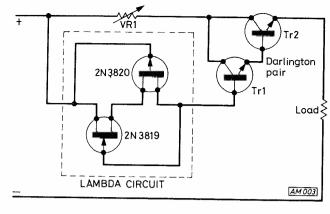
Fig. 3: A protection circuit using a lambda circuit as its over-current sensor.
