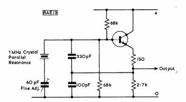
Fig. 64: A basic crystal oscillator circuit.
