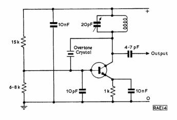
Fig. 65 : An overtone crystal oscillator circuit.
