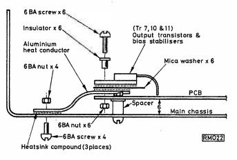
Fig. 6: Assembly details for output transistors and heat sink.
