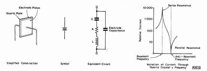
Fig. 63 : Features of a quartz crystal.
