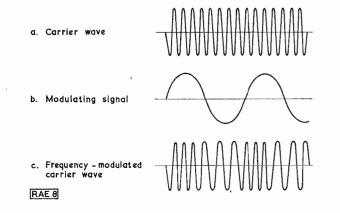
Fig. 59 : Frequency modulation of a carrier wave.
