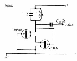
Fig. 4: A sinusoidal oscillator based on the lambda circuit.
