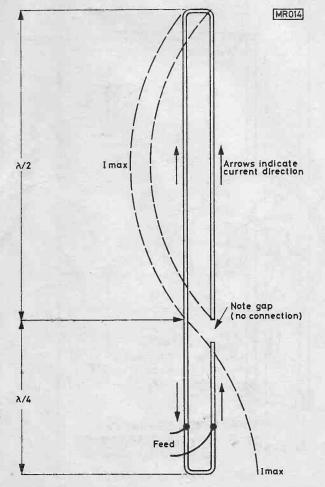
Fig. 1: The basic aerial, showing direction of current flow and phase reversal in matching stub.
