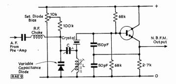
Fig. 60 : A typical n.b.f.m. oscillator circuit.
