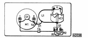
when the circuit is resonant at the frequency of excitation. Hence a maximum indication occurs at resonance and, since the tuned circuit is calibrated, it is possible to determine the frequency of excitation.
