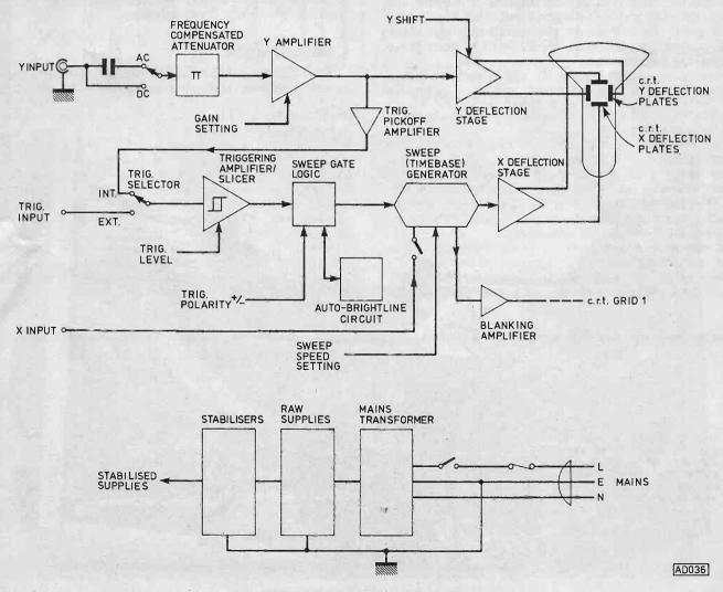
Fig. 2: Block diagram of the complete oscilloscope
