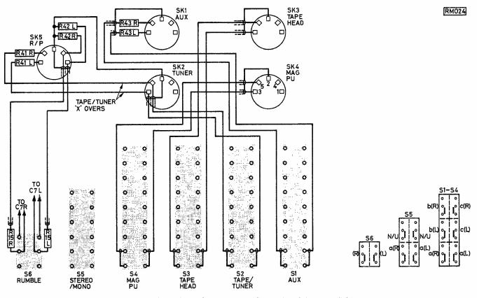
Fig. 7: Wiring details for the input sockets and push-button switch assembly. To avoid hum-producing earth loops, the cable screens must be connected only at the point shown. The photograph above shows the switch area in a prototype amplifier.
