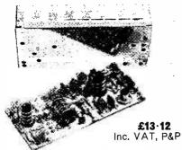
**TECHNICAL CHARACTERISTICS:** Output terminal for digital frequency meter; Antenna Impedance—75 to 300 Ohms; Frequency ranges 87.5 to 104MHz or to 108MHz; Sensitivity—0.9u V 26dB signal to noise ratio ±75kHz deviation; Intermodulation 80dB Image rejection—60dB; Tuning voltage—1V to 11V; Total gain—33dB; Intermediate frequency—10.7MHz; Power supply voltage + 15V; Power consumption 15mA; Dimensions 104 × 50mm.
