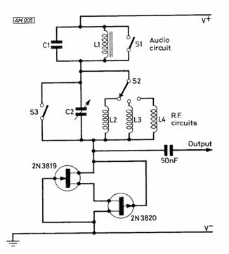
Fig. 5: An r.f. [a.f. signal generator using the lambda circuit.
