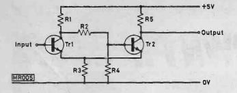
Fig. 2: A basic Schmitt trigger circuit using npn transistors.
