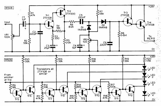
Fig. 1 (top): The circuit diagram of the buffer amplifier and rectifier. The rectified peak to peak voltage appears at the emitter of Trd.
