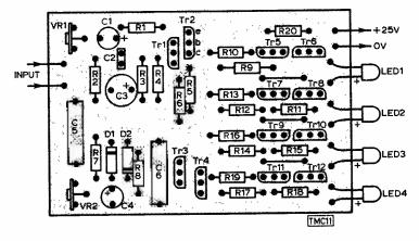
The current consumption of the circuit is approximately 25mA from a 25V supply. The display is bright enough to be clear in fairly strong daylight.
