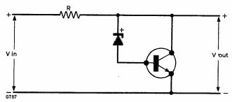
Fig. 2: Use of a shunt regulator transistor to relieve the load on the zener diode.
