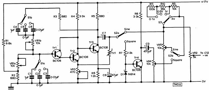
Fig. 3: Circuit diagram of the AF Signal Generator. The voltage follower circuitry surrounding IC1 may not be required (see text 'Construction').
