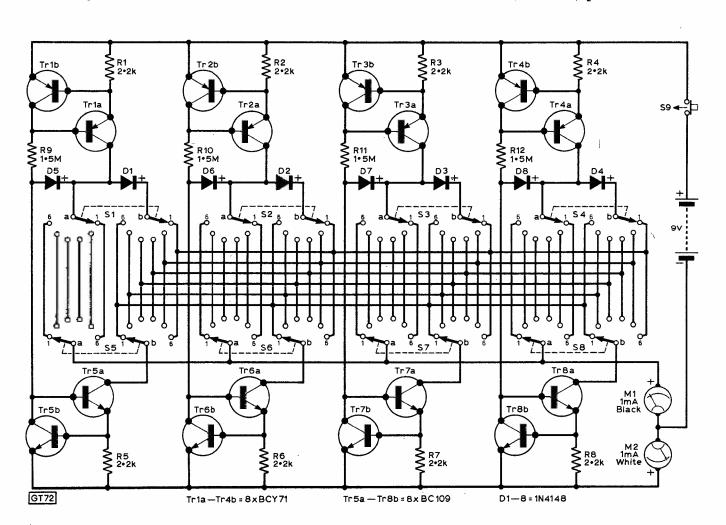
Fig. 1: The complete circuit diagram, showing the extensive use of constant current stages.
