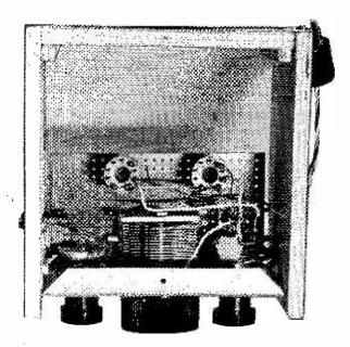
The finished preselector. If it is used with a different receiver an internal 9V battery can be incorporated, with an on-off switch on VR1.
