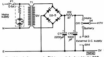
Fig. 4 (above): Power supply. C11 is mounted external to the PCB. Fig. 5 (below): The optional voltage follower circuitry. Simply leave these components off the PCB if not required.
