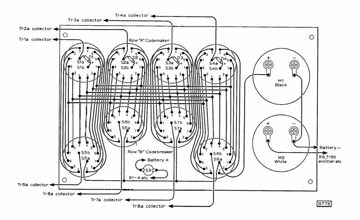
Fig. 2: The switch wiring, meter, and transistor connections.
