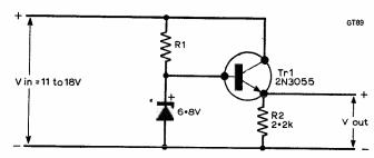
Fig. 4: The practical circuit so far with component values.
