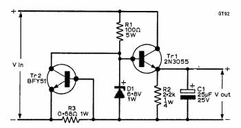
Fig. 7: The final circuit which Includes an overload sensing transistor
