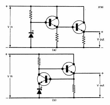
Fig. 5: above, a second transistor can be used in either of these circults.
