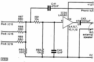
Fig. 5: Power amplifier schematic.
