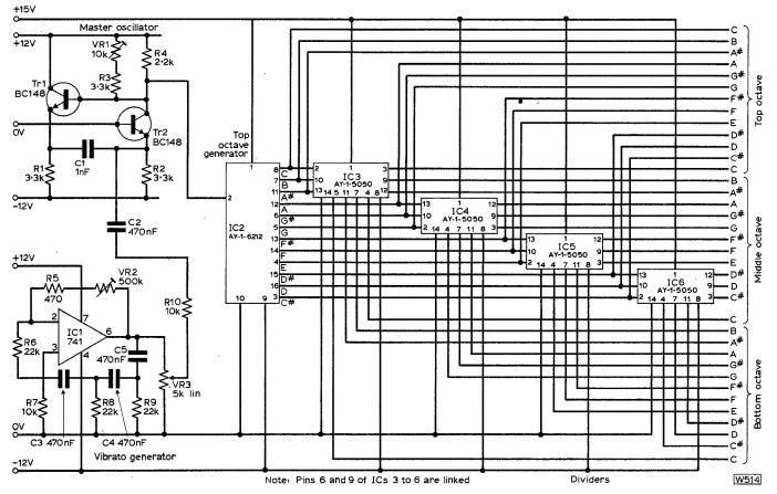
Fig. 6: Tone generator and divider circuits. When testing this section, take special notice of instructions in the penultimate paragraph (over page).
