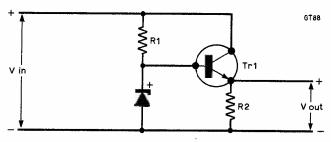
Fig. 3: The alternative series regulator circuit.
