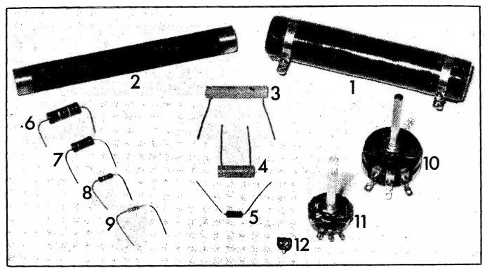
1. Wirewound Resistor 50W. 2. Carbon film resistor 30W. 3. Wirewound resistor 10W. 4. Wirewound resistor 5W 5. Wirewound resistor 2W. 6, 7, 8 and 9. Carbon film resistors, 2W, 1W, ½W and ½W. 10, 11
