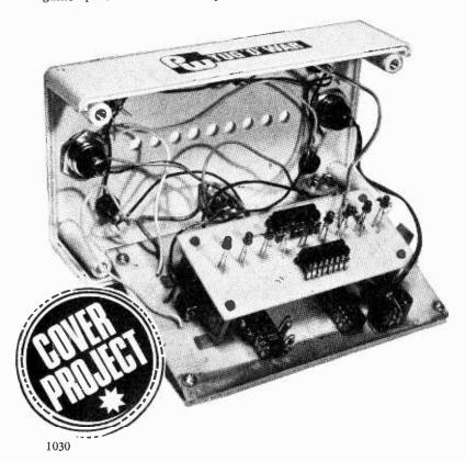
General interior photograph of the Tug-O-War, showing the board layout, interboard wiring and switch positioning.
