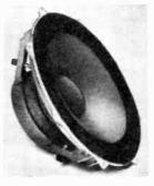
15" 14A/780. Bass unit on a rigid diecast chassis. Superior cone material handles up to 50 watts RMS, and is treated to give a smooth frequency response. Resonance 30 Hz. Hux density 360,000 Maxwells. Impedance at 1 kHz is 8 ohms. 3" voice coil.
